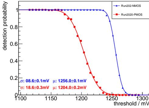
Figure 1: Exemplary response to the charge injection for RUN2020-NMOS (blue triangles) and RUN2020-PMOS (red squares). An s-curve is fitted to the data. The baseline is at 1 V.
