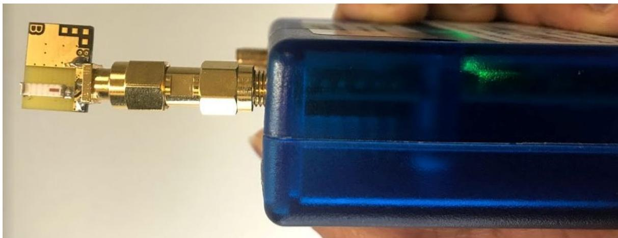
**Figure 5.8** – Transmitting antenna connected to the Mini VNA Tiny.
