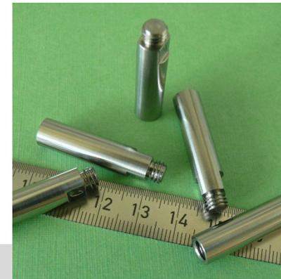
*Ø8×35 mm samples for exposure to flowing LBE.*
