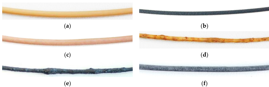
Figure 3. Images of extruded filaments (length 5 cm): (a) PEEK; (b) CF30 PEEK; (c) PEEK with 1.6 Vol% copper particles; (d) PEEK with 1.6 Vol% copper fibers; (e) PEEK with 2.3 Vol% CNT as extruded; (f) PEEK with 2.3 Vol% CNT postprocessed (grinded surface).
