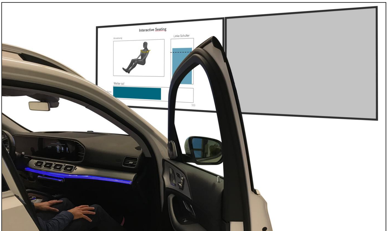
Figure 51: Illustration of the measurement setup. The right screen showed a video that was played during the ride (Dash Cam Tours, 2021), the left screen showed the user interface. Due to a missing copyright permission, the right screen was grayed out for this image.
