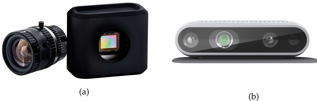
Figure A.1.: Photos of the used sensors. (a) Prophesee Evaluation Kit Gen3 HVGA-EM [436] with ATIS architecture [251]. (b) RealSense™ Depth Camera D435 [437].
