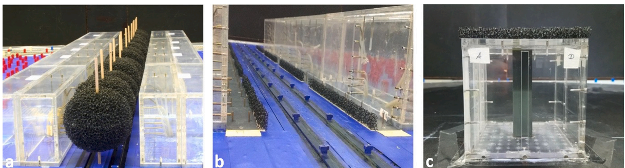
Fig. 6. Application examples of open porous foam processed to model (a) avenue-trees in an urban street canyon (Gromke and Ruck, 2007), (b) hedge-rows in an urban street canyon (Gromke et al., 2016), (c) roof greening of a building (Pappa et al., 2023).
