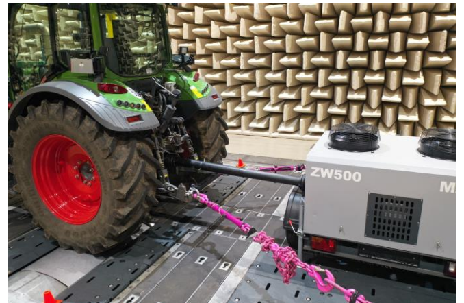
Figure 10. Tractor and eddy current brake on the test bench
