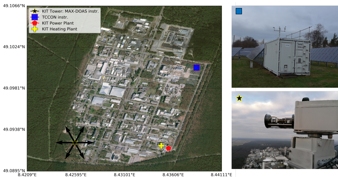
Figure 10.4: The map shows the locations of the TCCON station and MAX-DOAS instrument within the KIT CN map. The MAX-DOAS instrument is located at the top of the 200-m tall tower from IMK-TRO ( https://www.imk-tro.kit.edu/english/7791.php , last access: 02 October 2022.), the arrows represent the different azimuth angle directions used for collecting measurements. A heating and power plant operated by KIT are also shown on the map.
