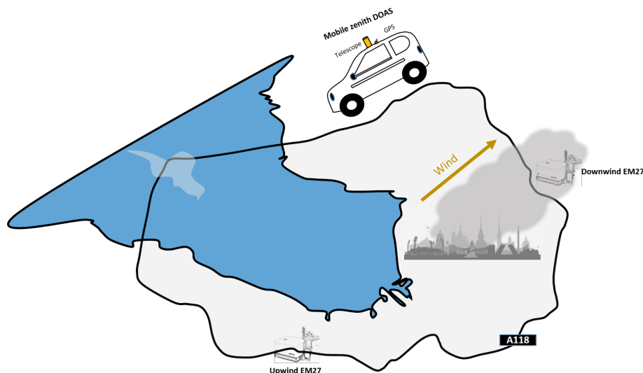
Figure 9.3: Map describing the positions of the instruments based on the wind direction
