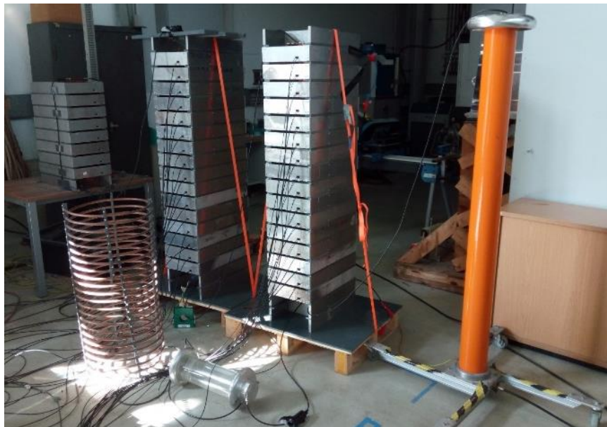
Fig. 2.2.1: 32-stage Marx generator connected to an artificial load.
