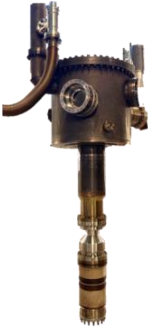
Fig. 1.1.2: Preparation of the first 2 MW 170/204 GHz coaxial-cavity short-pulse pre-prototype (collector is missing).
