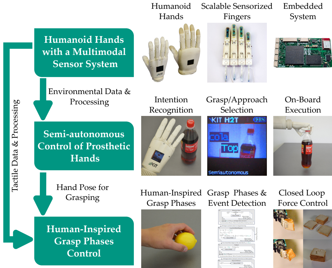
Figure 1.1.: Overview of the contributions in the thesis. Sensors perceive the state of the hand, robot/user as well as interactions with the environment. Based on the provided sensor information a semi-autonomous pre-grasp control scheme controls hand preshape and wrist orientation prior to grasping known objects. During the actual grasp, an automatic grasp-phases controller generates suitable finger motions and contact forces to grasp, hold and replace unknown objects.
