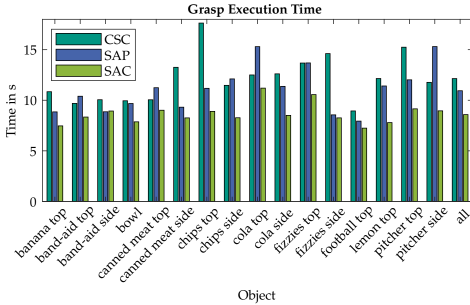
Figure 4.8.: Time required to execute the grasps on all ten objects and the overall grasp execution time in the three evaluated control strategies. Reprinted from (Starke, Weiner et al., 2022) with changes (CC BY 4.0).
