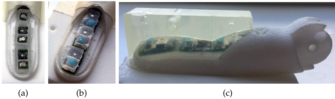
Figure 3.16.: (a) The molds for the silicone rubber casting process are placed directly into the finger. (b) The individual sensors have been cast in rubber. The next step is to cast the remaining finger pad area in rubber. (c) The result of the casting process of the finger tip and one half of the used mold is shown. A silicone canal is used to inject silicone rubber into the molds. Reprinted from (Weiner et al., 2019) without changes (CC BY 4.0).
