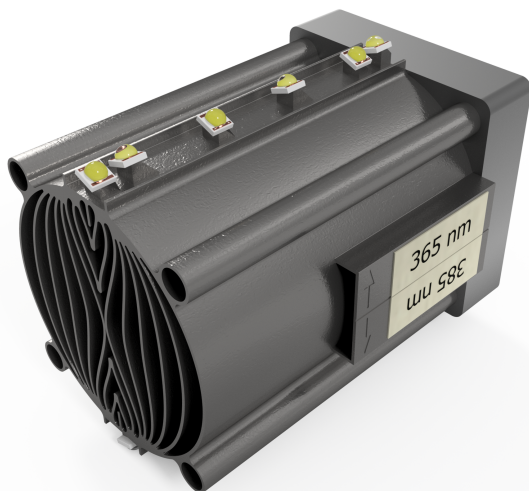
Figure 7.5.: Rendering of a CAD model of the LED light source modules shining their light into the optics module of the developed isophotonic photoreactor. The small inclined pillars on which the SMD LEDs are placed ensure the derived optimal inclination and positions of the LEDs resulting in an isophotonic reaction volume.
