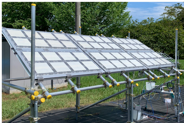
Figure 2.10.: Panel like production photoreactor with photoelectro chemical photocatalyst splitting water to hydrogen and oxygen. Reprinted with permission from Springer Nature, [23], Copyright 2021.
