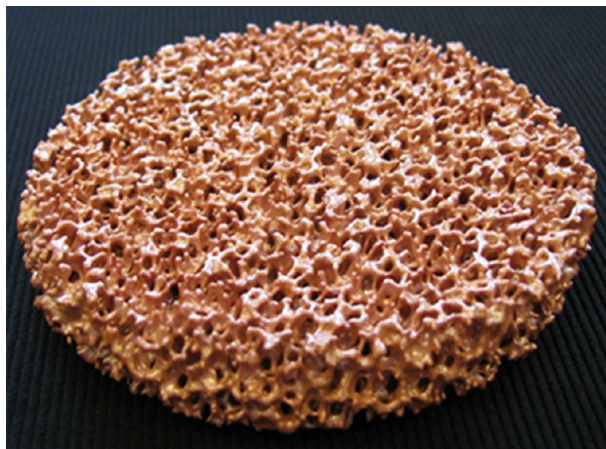
Figure 2.4.: Photograph of a reticulated foam made from ceria and employed in a high temperature redox cycle splitting carbon dioxide to carbon monoxide and oxygen. Reprinted with permission from [76]. Copyright 2012 American Chemical Society.
