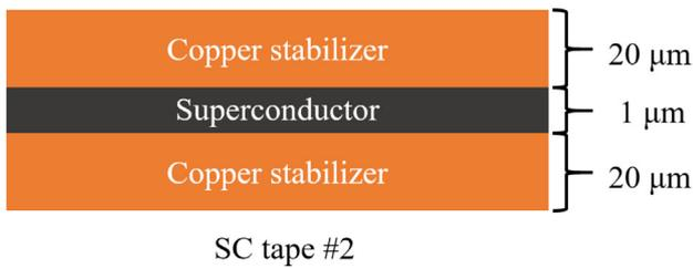
**Fig. 3.** Schematic of the modeled HTS bridge (SC tape #2) cross-section (not to scale).
