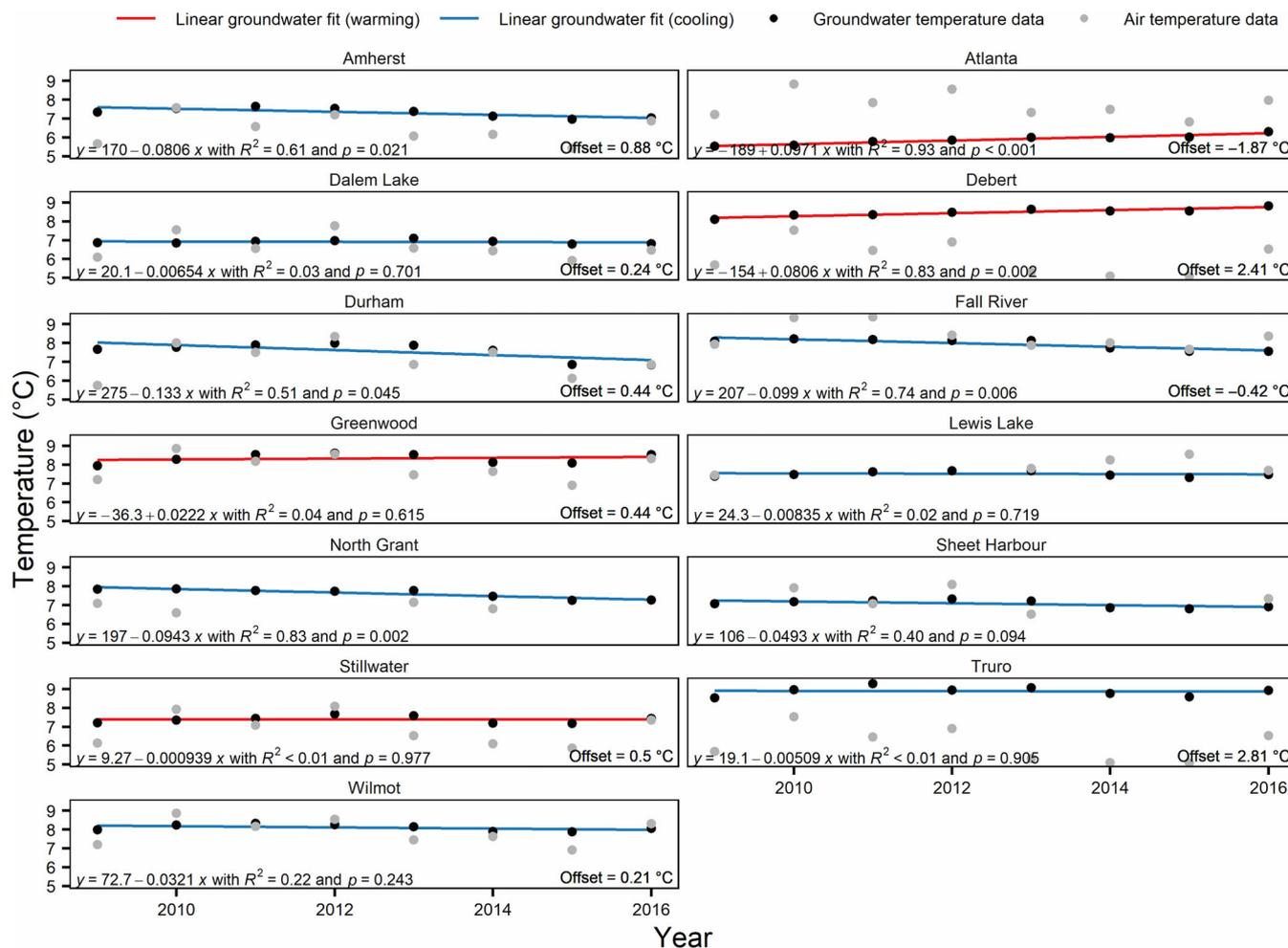
**FIGURE 4** Mean annual groundwater and air temperatures (points) for observation wells with continuous data from 2009 to 2016 fitted with linear regressions (lines) versus year for groundwater temperature. Offsets shown in text in each pane were calculated by subtracting the mean air temperature from the mean groundwater temperature from 2009 to 2016.
