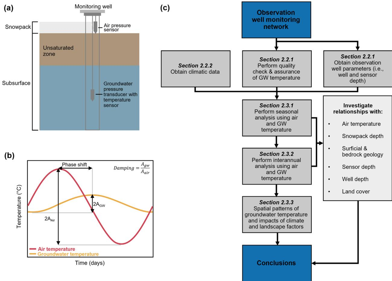
**FIGURE 2** (a) A conceptual diagram of an instrumented monitoring well. (b) Subsurface damping and lagging of an air temperature signal. (c) A flow chart indicating the data analysis approach.
