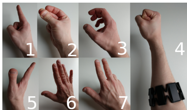
Figure 2. Gestures used to test our classification procedure. Top row, left to right: point, snap, open. Bottom row, left to right: wave out, wave, count. Right column: fist with Myo Armband attached to the forearm.
