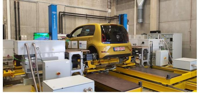
Figure 4. Mounted VUT at the ViL test bench of the KIT-FAST.
