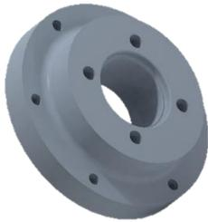
Figure 9. Rendering of the wheel hub adapter for mounting the VUT at the ViL.
