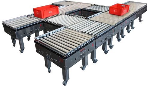
Figure 2.2: Conveying network of FlexConveyor modules (Seibold et al. 2013).
