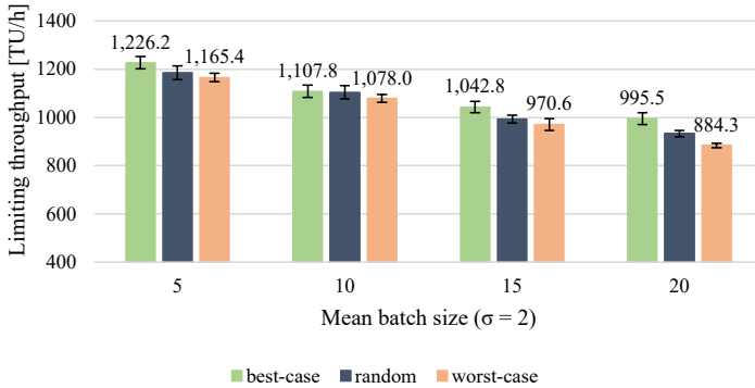
Figure 8.4: Limiting throughput depending on arrival sequence for selected batch sizes ( s = 1 ).
