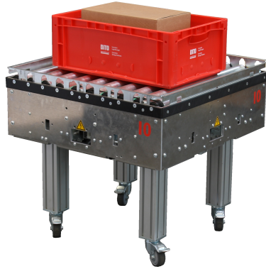
Figure 3.3: FlexConveyor module (Karlsruhe Institute of Technology: Institute for Material Handling and Logistics 2009).
