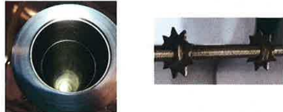
Figure 3. Electrode system of a conventional ESP with grounded tube and HV star-form electrodes
