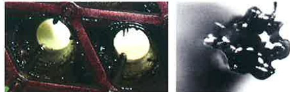
Figure 1. Electrode system of a space charge ESP with high velocity nozzles and HV needle electrodes
