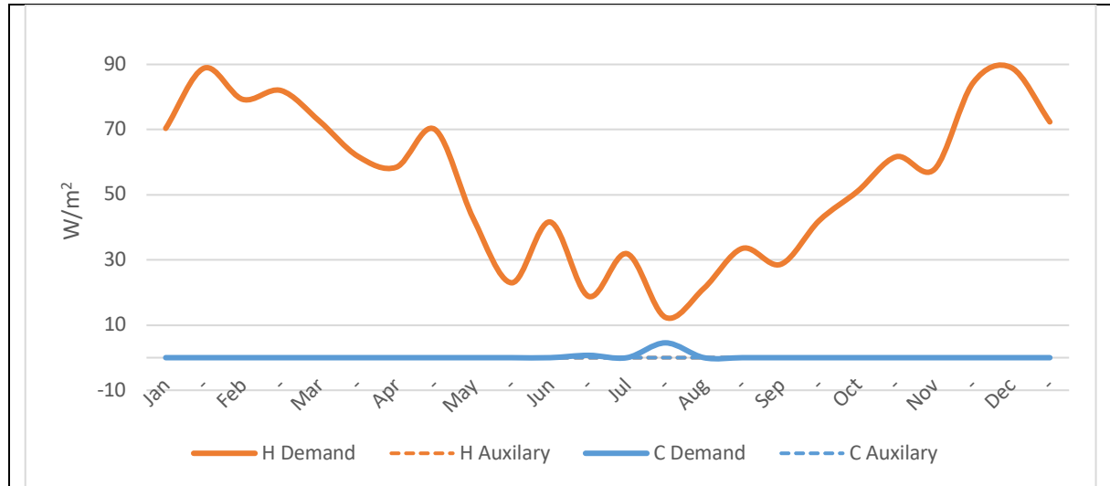
Fig. 5.53 Monthly cumulative heating demand, heating auxiliary, cooling demand and cooling auxiliary – BAPV (W/m 2 ), Geometrical setup and boundary condition in table 5.42
