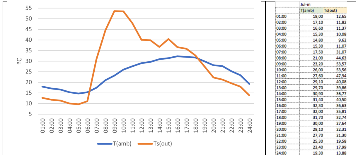
Fig. 5.21 Outside air and surface temperature of component – boundary condition table 5.18
