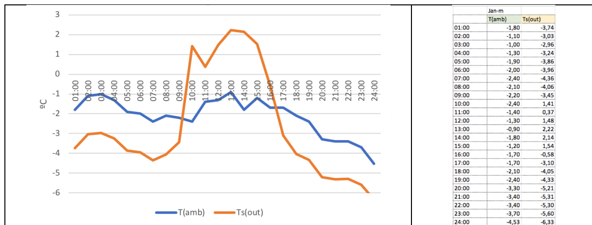
Fig. 5.19 Outside air and surface temperature of component – boundary condition table 5.18
