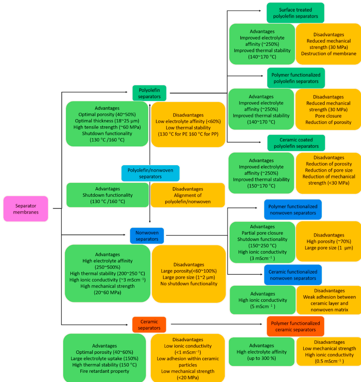
Fig. 5. Categorization of the evolution of separators and the overall advantages and disadvantages of various types of separators.
