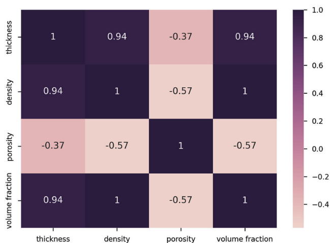
Figure 4. Heatmap showing the correlation between different target physical properties. The low variance and weak correlation of porosity with other properties explain the low R^2 score in predicting the porosity information of SEI configurations.
