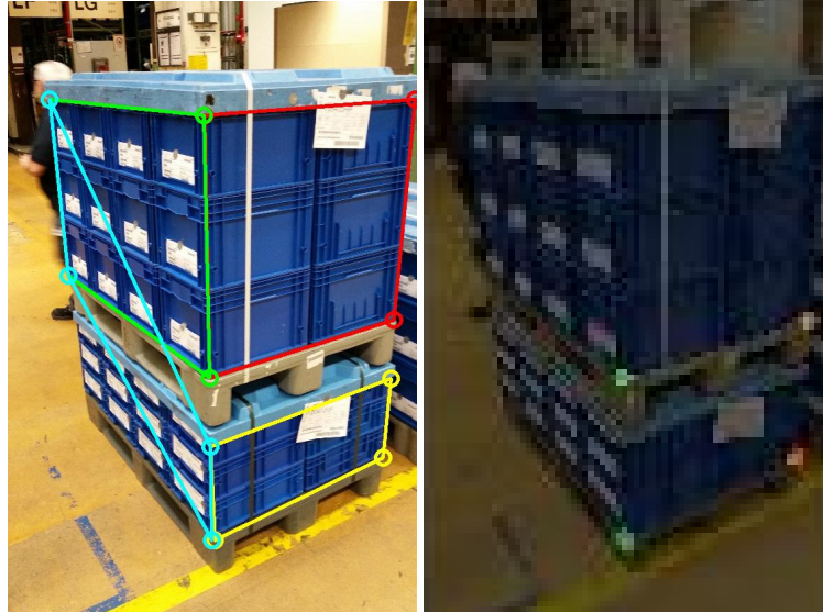
Figure 6.8: False assignment of object corners to objects and color-encoded embedding values of bottom right corners.
