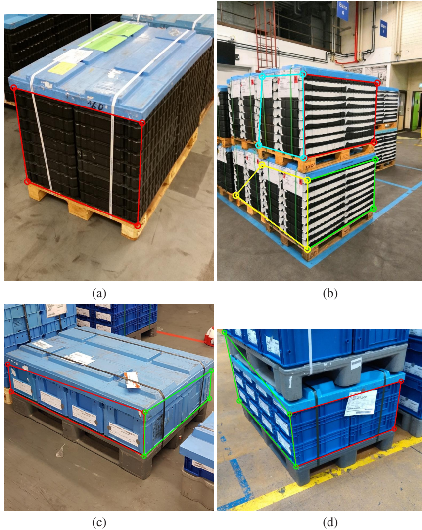
Figure 6.7: Examples for cases in which TetraPackNet does not segment all transport unit sides correctly. (a) One transport unit side is not found at all. (b), (d) A corner point of an adjacent background transport unit side is mistakenly employed. In (d), the type of corner point is mistaken, too (top left instead of bottom left corner). (c) Corner points are misplaced by a few pixels onto the transport unit lid instead of the packaging unit corner.
