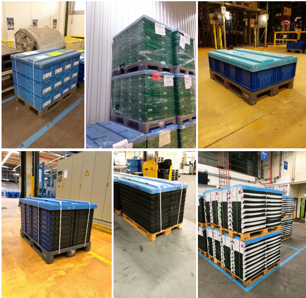
Figure 4.3: Examples from our dataset of 1,000 images. Top row: KLT package unit type. Bottom row: Tray package unit type.
