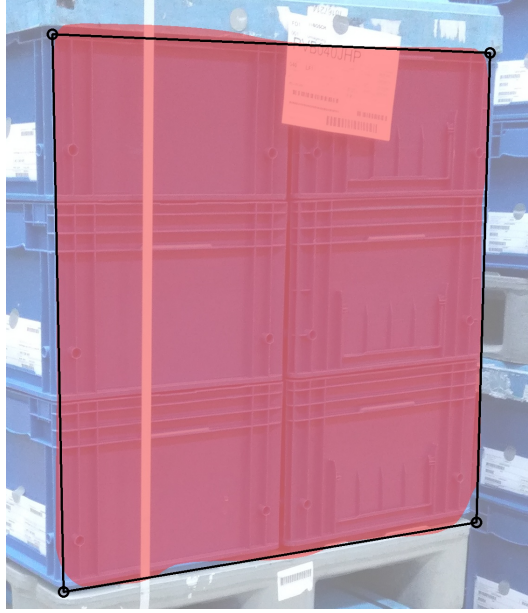
Figure 4.2: Illustration of the transport unit side mask simplification performed as sub-step of the Information Consolidation process. The detected transport unit side region is indicated in red. The four black dots indicate the four corners output by the post-processing optimization algorithm.
