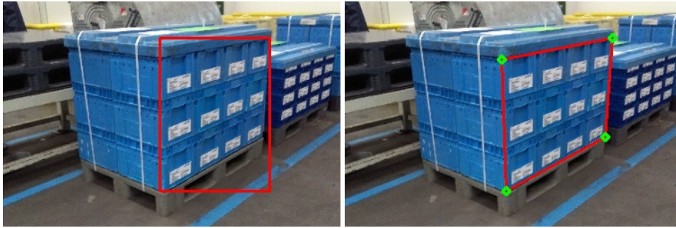
Figure 6.1: Sample annotations. Left: Bounding box annotation. Right: Four-corner-based annotation. The example image is taken from our use-case-specific dataset.
