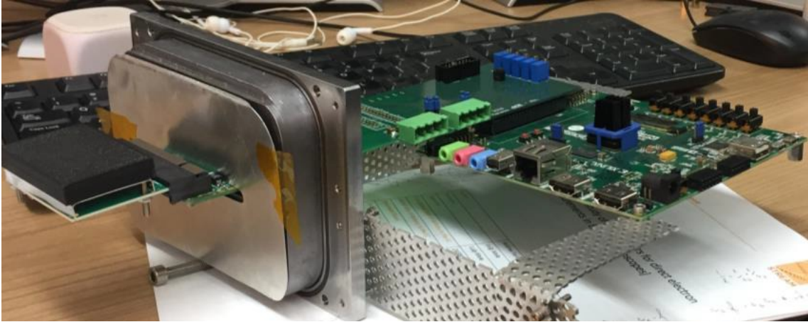
Figure 2.41: PCB interface used for communication between HPIXEL and FPGA after it has been placed in the lid of the vacuum chamber of the TEM.
