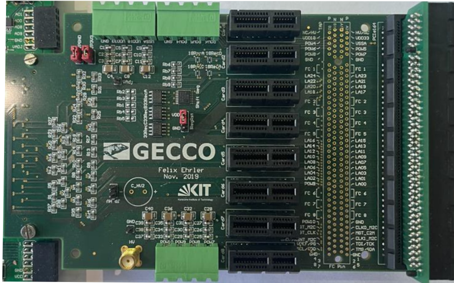
Figure 3.23: GECCO-board used to communicate the HINT sensor with the FPGA.
