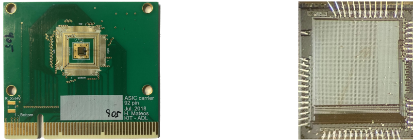
(a) PCB carrier with HPIXEL sensor glued and wire bonded. (b) Close up of the HPIXEL glued and wire bonded to the PCB carrier.
