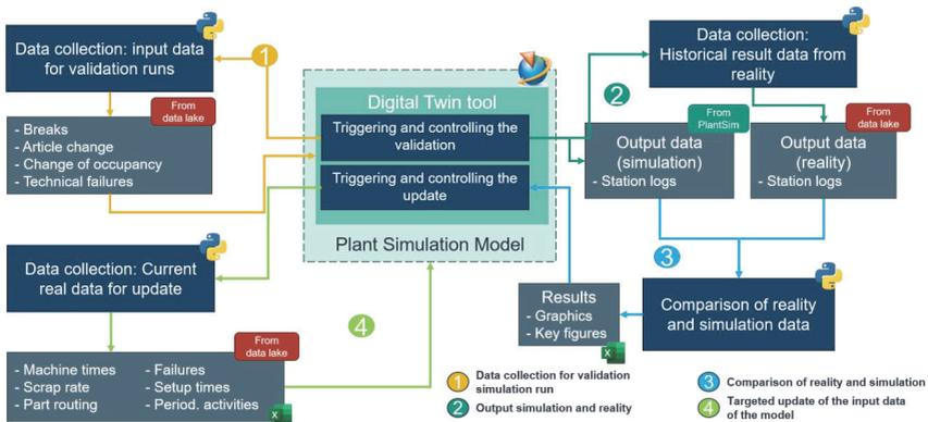
Figure 5-9 Sequence of validation based on A\_Le Louarn (2021)
