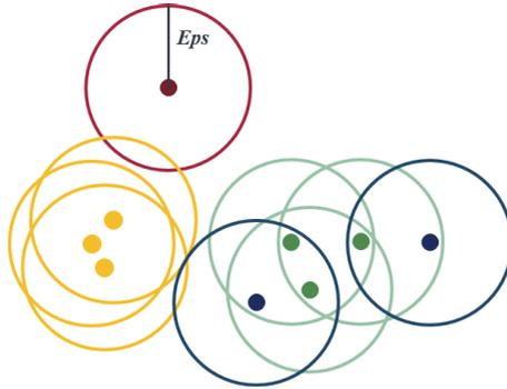
Figure 2-13 Visualization clustering with the DBSCAN algorithm
