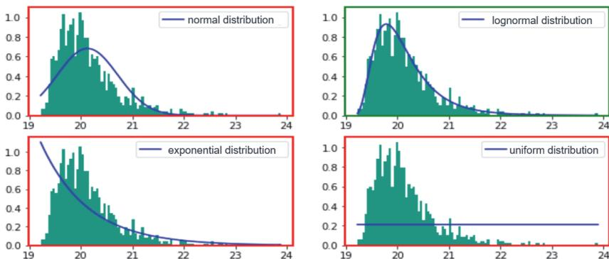
Figure 4-14 Histogram with four different distribution functions. The lognormal distribution fits best (A\_Haizmann 2020)
