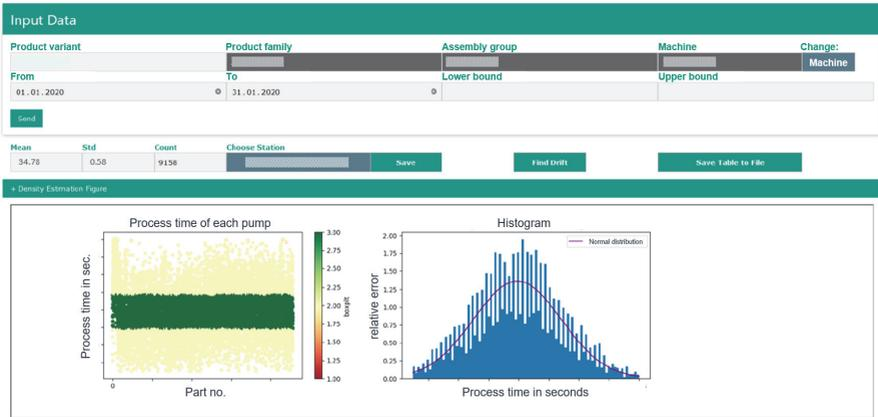
Figure 5-13 Web application with a scatter plot for a product variant at a station and fitted normal distribution according to A\_Haizmann (2020, p. 77)
