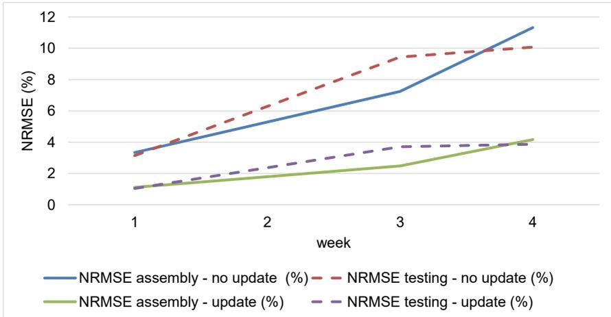
Figure 6-2 Development of the accuracy of the Digital Twin of line 1 with and without update
