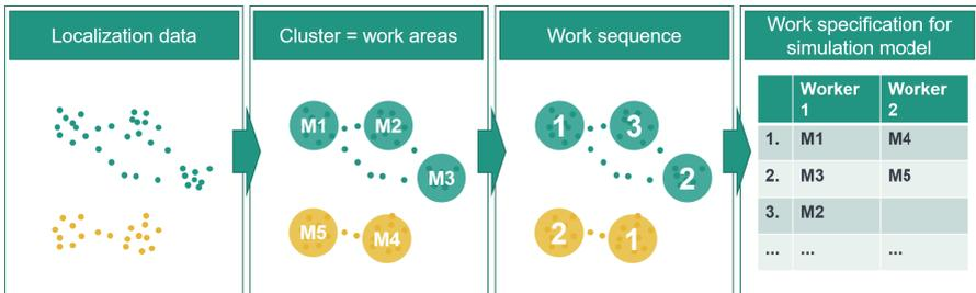
Figure 4-16 Schematic flow of the determination of the work processes in the production system
