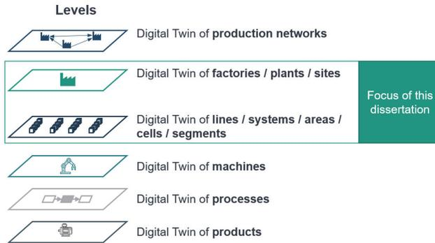
Figure 2-8 Possible Digital Twins on the structuring levels of production, based on (Westkämper 2007, p. 11; Wiendahl et al. 2007)
