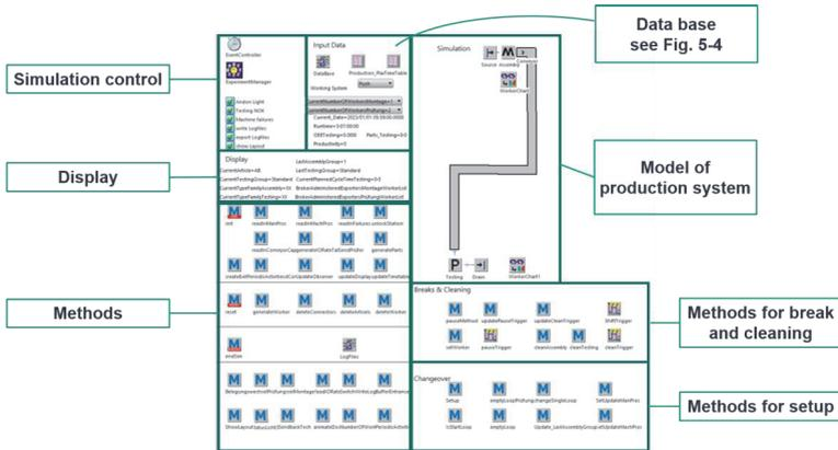
Figure 5-3 Model view in Plant Simulation (2D)
