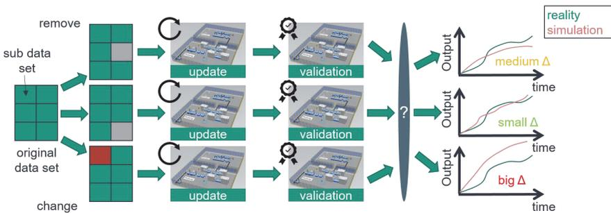
Figure 6-8 Schema of sensitivity analysis
