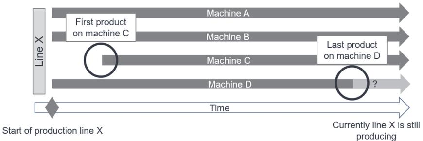
Figure 4-18 Schematic detection of commissioning and end of operation of machines A-D in line X
