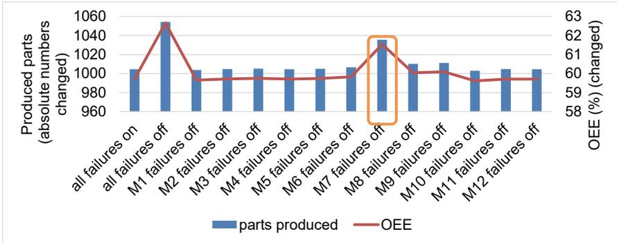
Figure 6-23 Influence of failures on different machines on the performance of the production system
