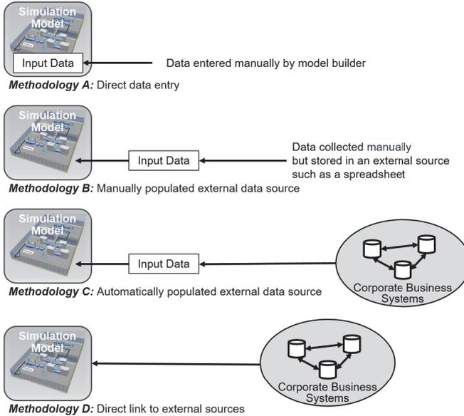
Figure 2-7 Ways to enter data into the simulation model (Robertson & Perera 2002)
