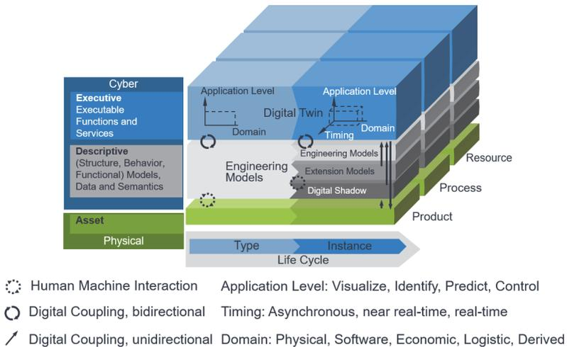
Figure 3-1 Structure model for Digital Twins according to Lechler et al. (2020)
