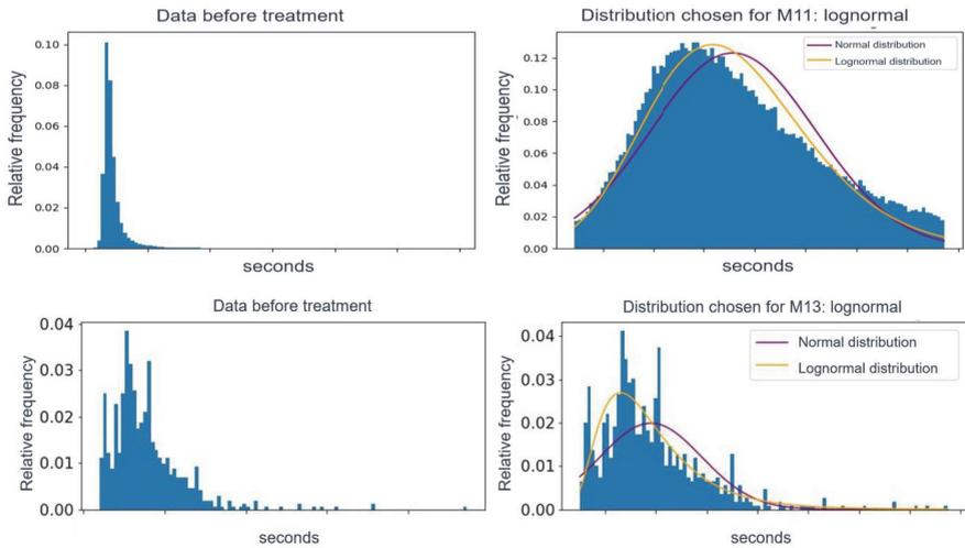
Figure 5-14 Example of distribution fitting at machines 11 and 13 for one product variant
