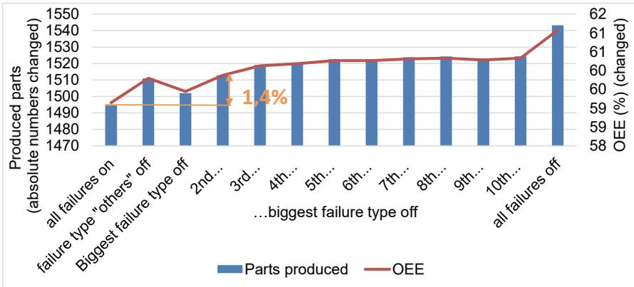
Figure 6-24 Influence of the most important failure types of machine 7 on the performance of the production system
