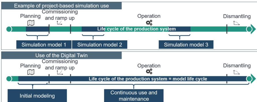
Figure 1-1 Use of conventional simulation models versus the use of a Digital Twin
