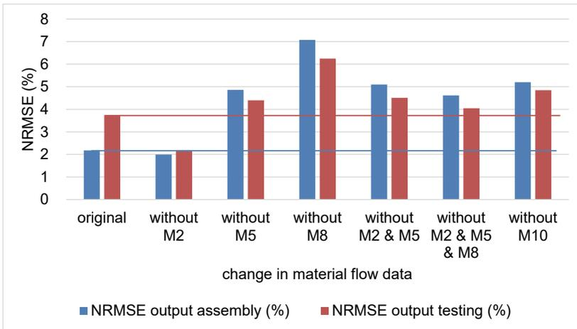
Figure 6-16 Effect of changes in material flow data on accuracy of the Digital Twin
