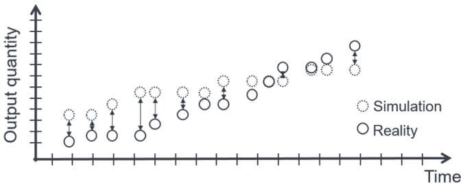
Figure 4-7 Illustration of the NRMSE calculation in the industrial use case (Overbeck et al. 2023)
