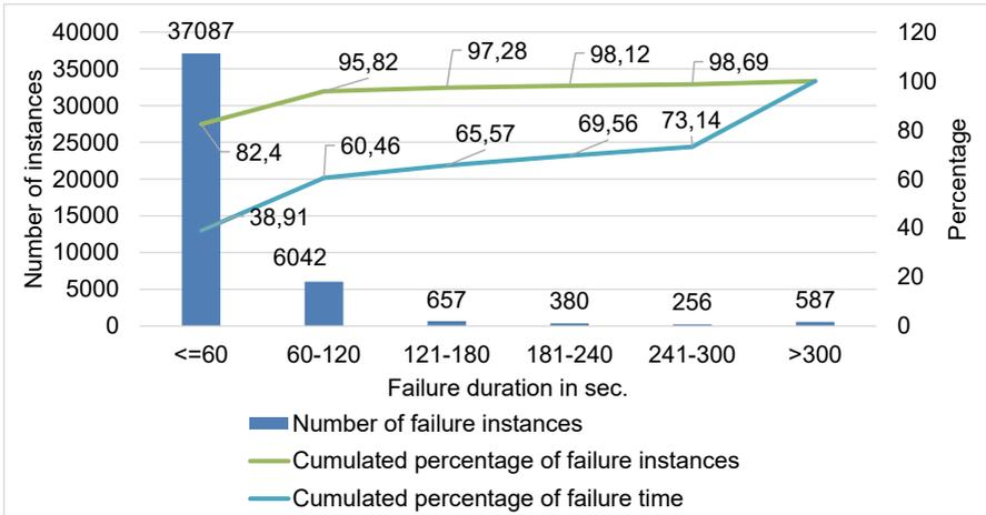
Figure 5-10 Distribution of failure durations of the automatically recorded failure messages
