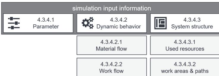
Figure 4-13 Structure of simulation input calculation
