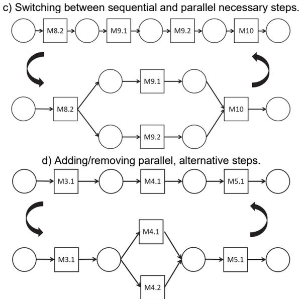
Figure 5-19 Examples of observed changes in the production process (Overbeck et al. 2023)
