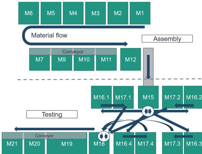
Figure 5-1 Schematic representation of the assembly and testing & completion subsystems
