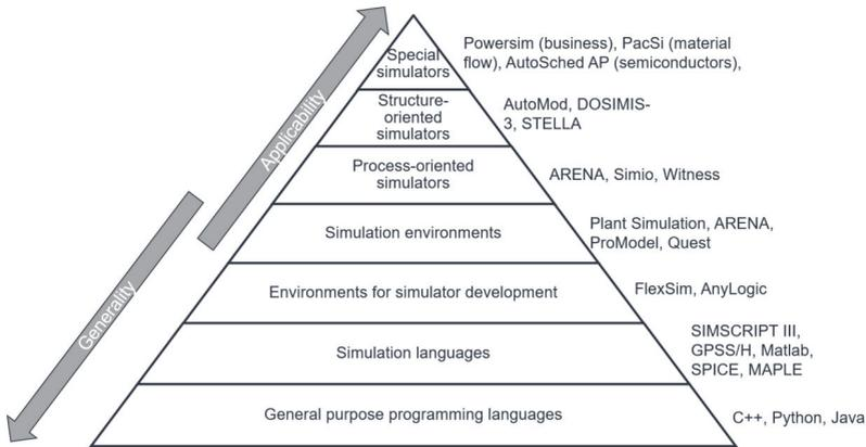
Figure 2-11 Classification of simulation tools for production and logistics, actualized and based on Eley (2012, p. 10) and Wenzel (2008)
