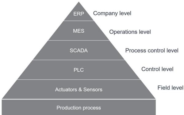
Figure 2-12 The automation pyramid (Siepmann 2016)
