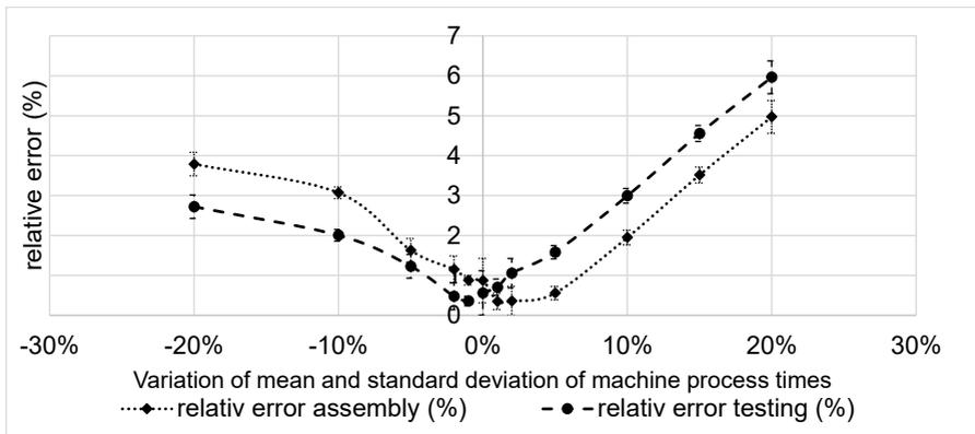
Figure 6-9 Change in relative error when varying mean and standard deviation including the 95% confidence interval
