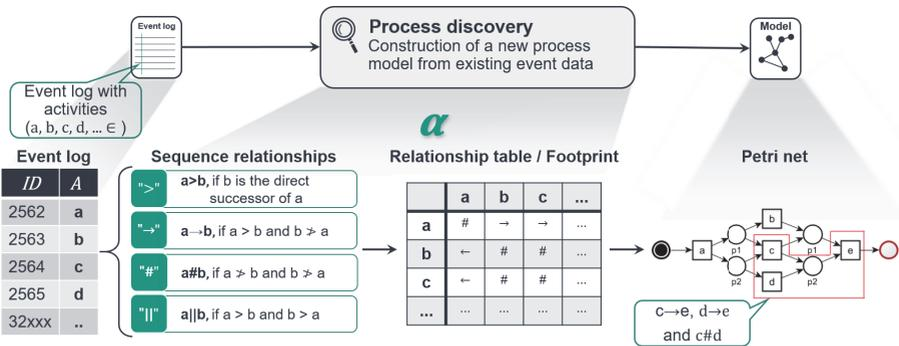
Figure 2-14 The alpha algorithm
