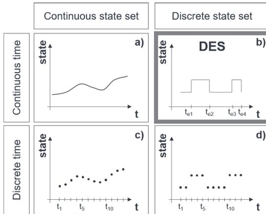
Figure 2-4 Classification of simulation models according to time and state set
