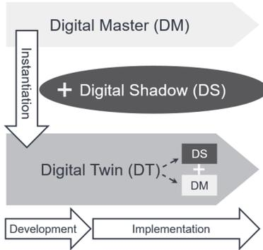
Figure 2-2 Components of the Digital Twin according to Stark et al. (2017)
