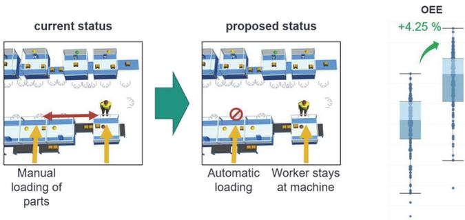
Figure 6-25 Example for the evaluation of hardware changes in the production system
