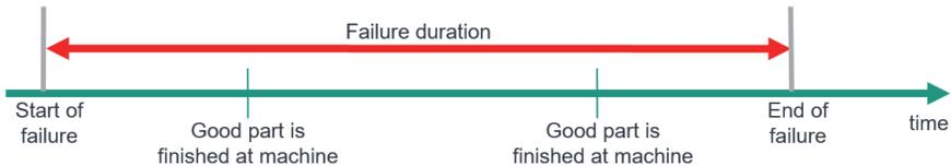
Figure 5-15 Identification of pseudo failures by comparison with machine protocol
