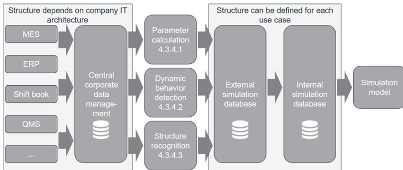
Figure 4-12 General procedure for determining the simulation input information
