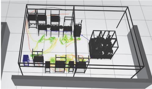
Figure 5-21 Visualization of recorded worker movements in the learning factory<sup>7</sup>
