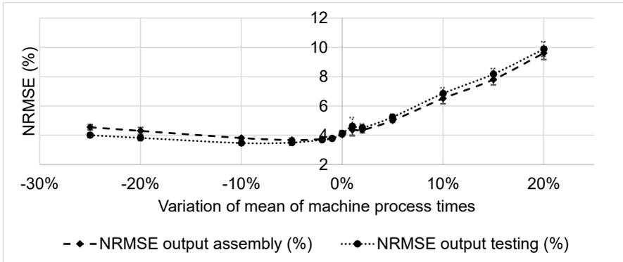
Figure 6-11 Change of average NRMSE when varying the mean value including the 95% confidence interval (Overbeck et al. 2023)
