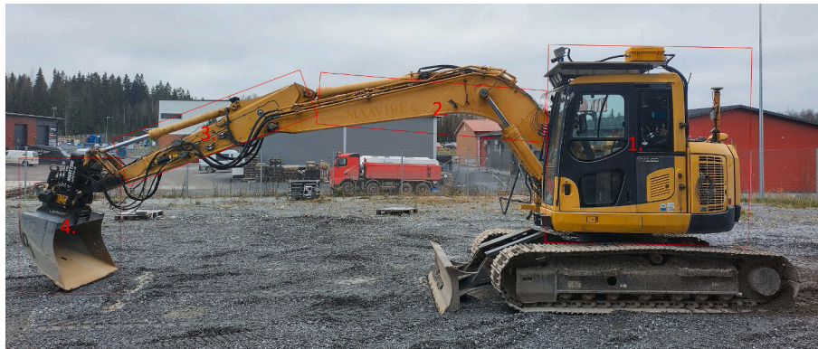
Fig. 3. Excavator used in data collection. In picture, cabin (1), boom (2), arm (3), and bucket (4) are highlighted with red boxes [8]. (For interpretation of the references to color in this figure legend, the reader is referred to the web version of this article.)
