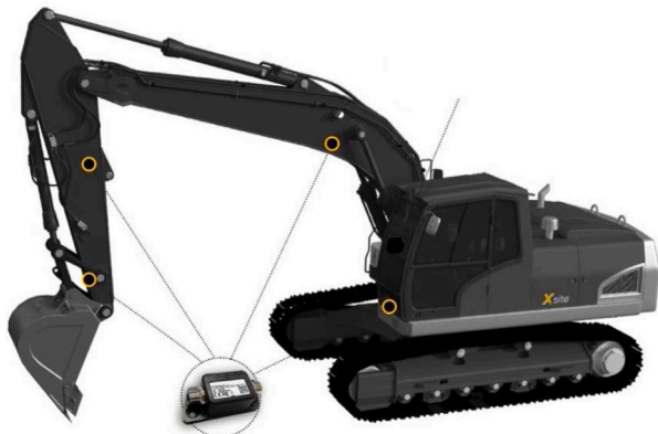
Fig. 5. Configuration of IMUs on an excavator.
