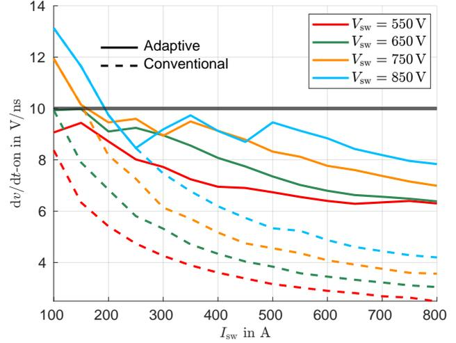
**Fig. 13:** Comparison of turn-on  $dv/dt$
