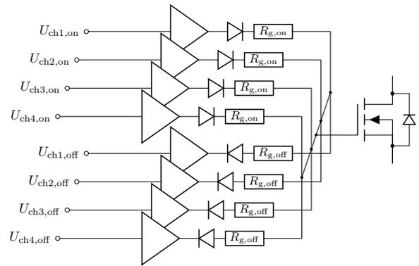
**Fig. 1:** Simplified schematic of the proposed gate-driver
