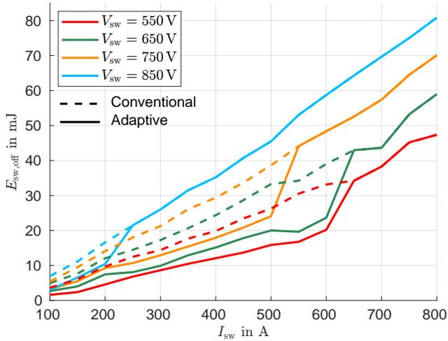
**Fig. 10:** Comparison of turn-off energies
