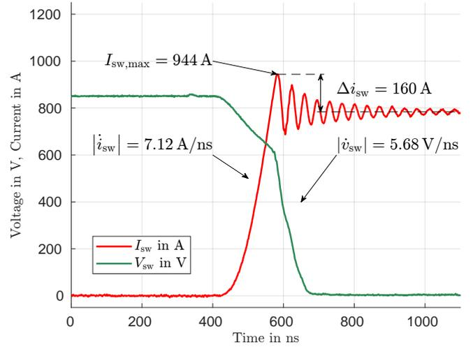
**Fig. 4:** Turn-on transient for  $R_{G,on} = 2.8 \Omega$
