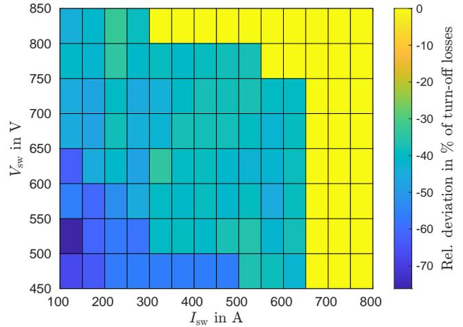
**Fig. 8:** Relative improvement of turn-off losses
