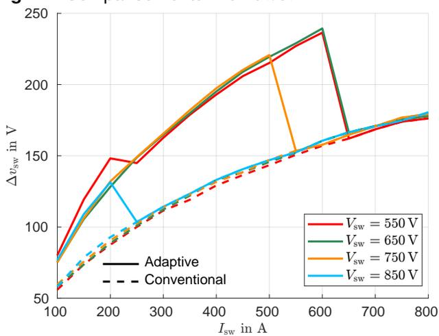
**Fig. 14:** Comparison of turn-off  $\Delta v_{sw}$
