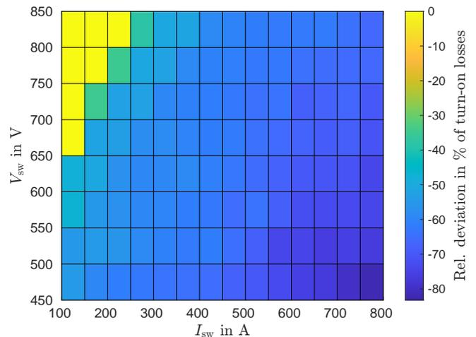
**Fig. 9:** Relative improvement of turn-on losses
