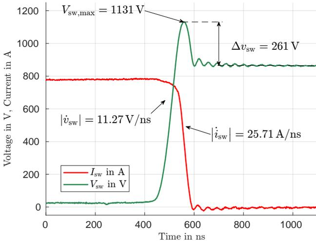
**Fig. 3:** Turn-off transient for  $R_{G,off} = 2.8 \Omega$
