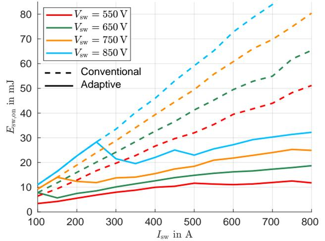
**Fig. 11:** Comparison of turn-on energies
