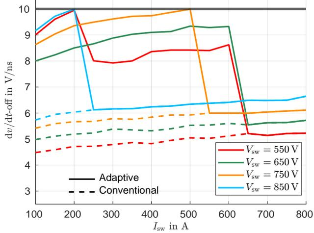
**Fig. 12:** Comparison of turn-off  $dv/dt$
