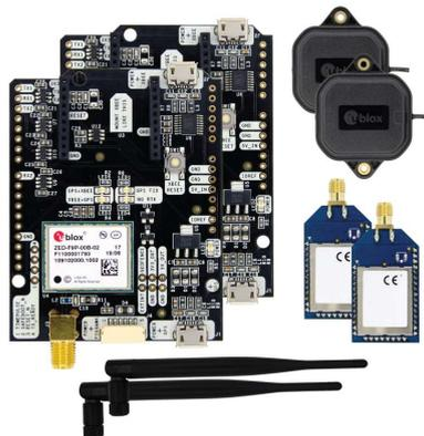
Figure 4.1: The *simpleRTK2B Starter Kit LR* from ARDU SIMPLE [44], which is comprised of two GNSS development boards (top left), dual-band GNSS antennas (top right), XBEE radio modules (bottom right), and radio antennas (bottom).
