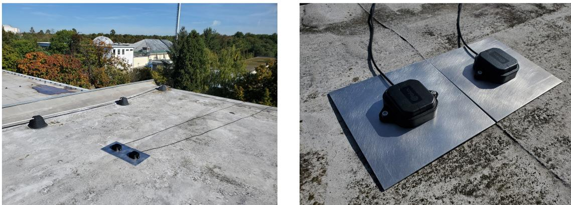
Figure 4.4: *Left*: The GNSS antennas are placed next to each other on the selected roof location. *Right*: Close-up of the GNSS antennas, mounted on custom  $15 \times 15$  cm aluminium plates.
