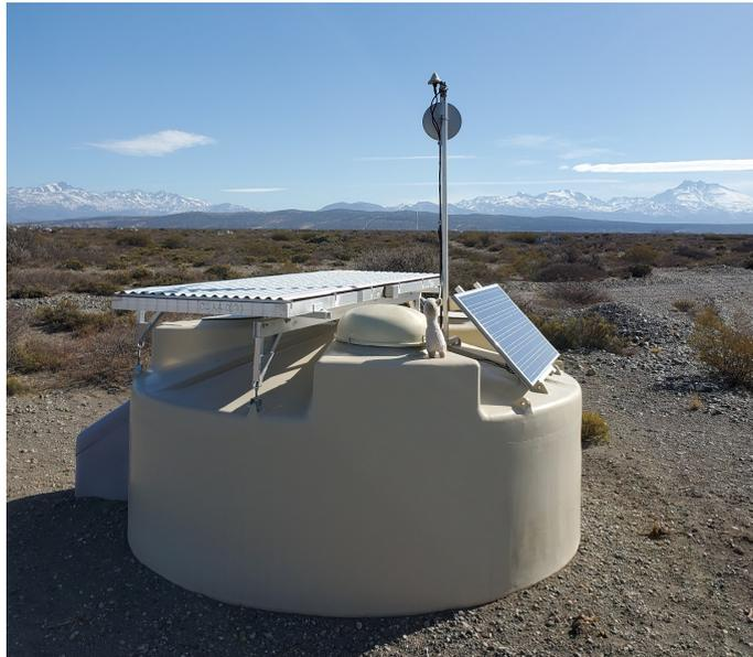
Figure 2.5: Photo of a Surface Detector (SD) station featuring a solar panel, communications antenna and surface scintillator detector (SSD) panel on top of the water Cherenkov detector (WCD). The electronics are encapsulated in the dome.
