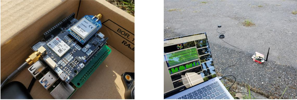
Figure 4.3: Photographs of the setup evaluating the GNSS boards. *Left*: Close-up of the base receiver while it is obtaining a position fix. *Right*: Laptop running the *u-center* software, monitoring the rover receiver and antenna placed on the ground outside the institute building.
