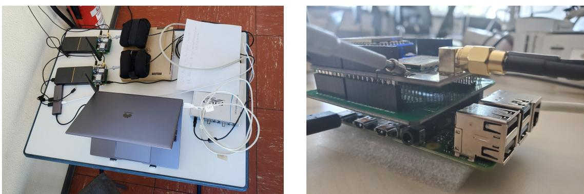
Figure 4.6: *Left*: Top-down view of the measurement setup. On the left are both GNSS boards, connected to the laptop in the lower center. The oscilloscope is visible on the right and also connected to the laptop. The oscilloscope probes are in the top center, connected to the boards and the oscilloscope. *Right*: Close-up of an oscilloscope probe making contact with the time pulse pin of the ARDUSIMPLE board.
