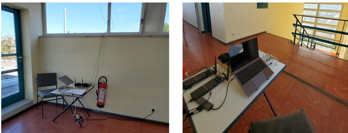
Figure 4.5: Pictures of the time-pulse measurement setup in the room below the roof location. Antenna cables are routed through the windows and the devices are powered by a power outlet.
