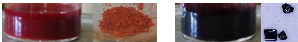
Figure 32. Visual appearance of Mbqn-(OH) 2 (left) and [CoCl 2 (MbqnO)] (right) in DMF solution as well as solid state highlighting the colour change characteristic for the complexation reaction in which the ligand reacts to a radical species. [28]
