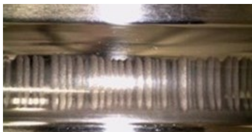
Fig. 2: Corrugated patterns at the raceway
