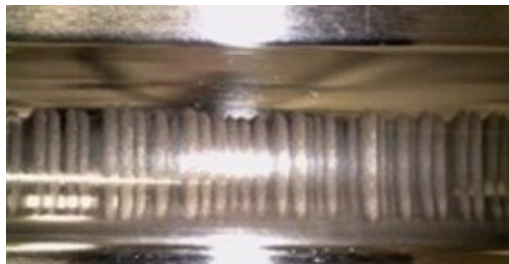
Fig. 2: Corrugated patterns at the raceway
