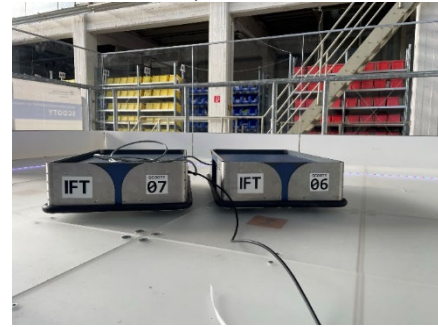
Figure 5.: Two omnidirectional robots, Scooty 06 and Scooty 07 , driving as a cooperative transportation group. A joystick is used to communicate the OCP to both robots. The distance of the robots is 100mm.
