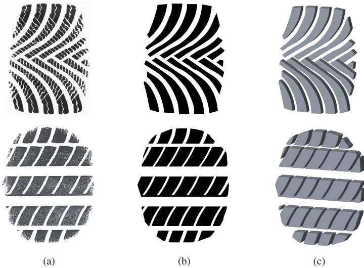
Figure 3.7: Transformation process from paper and ink to CAD geometry
