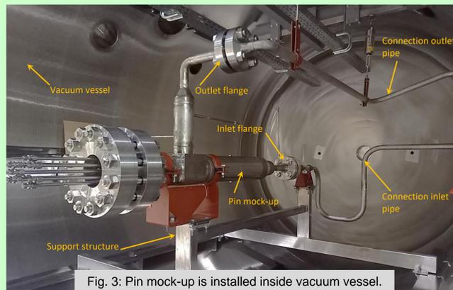
Fig. 3: Pin mock-up is installed inside vacuum vessel.
