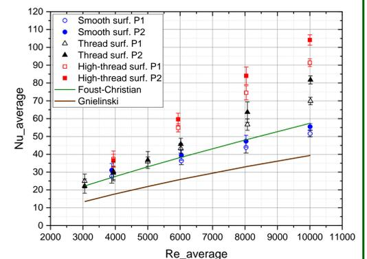
Fig. 11: Nu numbers obtained for the 3 different surfaces of Tube-3 (P1: Position1 & P2: Position2).
