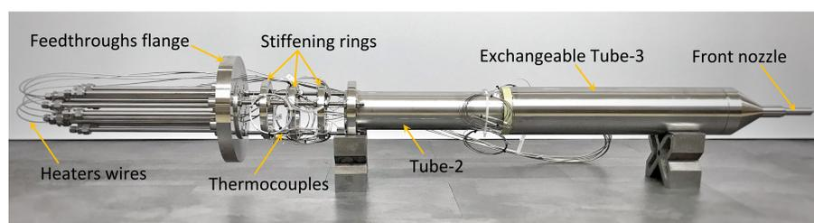
Fig. 6: The insert assembly with smooth-surface Tube-3.
