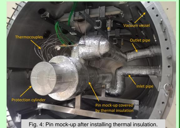
Fig. 4: Pin mock-up after installing thermal insulation.
