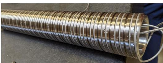
Fig. 7: Installing the coiled heaters on of Tube-1.
