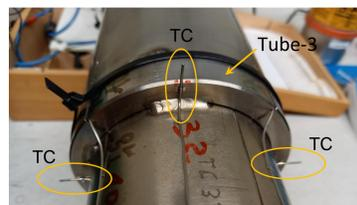
Fig. 8: Four TCs for helium bulk temperature.
