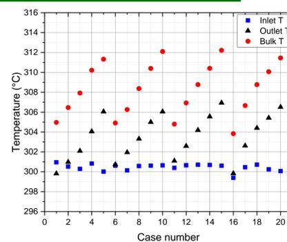
Fig. 9: Inlet, outlet & bulk helium T for smooth-surface Tube-3.
