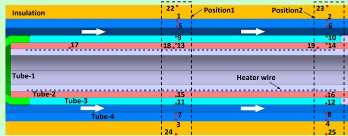
Fig. 2: The tubes & thermocouples TCs (numbers indicate TCs locations).
