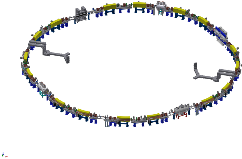
Figure 2.1: CAD drawing of the KARA storage ring. The storage ring consists of 16 dipole magnets (yellow) used for deflecting the electron bunches and 40 quadrupole magnets (brown) to focus the electron bunches. Image courtesy: Ursula Herberger.
