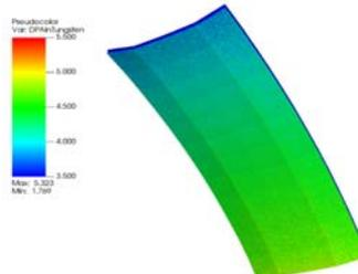
Fig 5: Neutron induced damage in tungsten [DPA/FPY]
