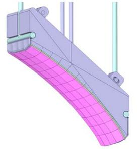
Fig 3: Detailed model of the upper limiter
