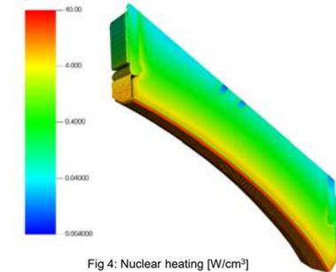
Fig 4: Nuclear heating [W/cm<sup>2</sup>]
