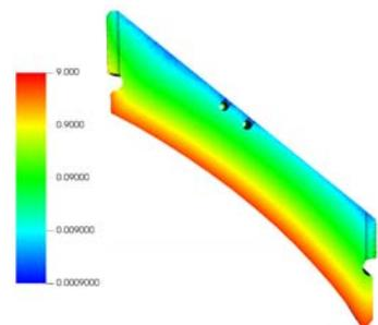
Fig 6: Neutron induced damage in Eurofer [DPA/FPY]
