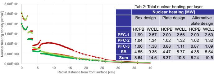
Fig 2: Radial dependence of the nuclear heating for different analyzed cases using simple upper limiter model
