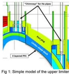
Fig 1: Simple model of the upper limiter
