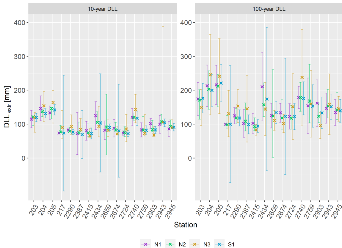
Figure 8. The 100-year and 10-year DLL_{extr} values obtained from extrapolated statistical models (2071–2100) with parameter estimation method MLE.
