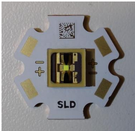
Figure 2 (a) Kyocera SLD element
