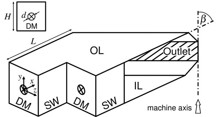
**FIGURE 7.** GEOMETRY OF TWO GENERIC SHC SECTORS. DM: DOME, SW: SIDEWALL, OL: OUTER LINER, IL: INNER LINER.
