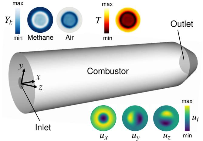
**FIGURE 4.** COMPUTATIONAL DOMAIN OF THE SINGLE-BURNER AND INLET PROFILES FOR SPECIES MASS FRACTIONS, TEMPERATURE AND VELOCITY COMPONENTS.
