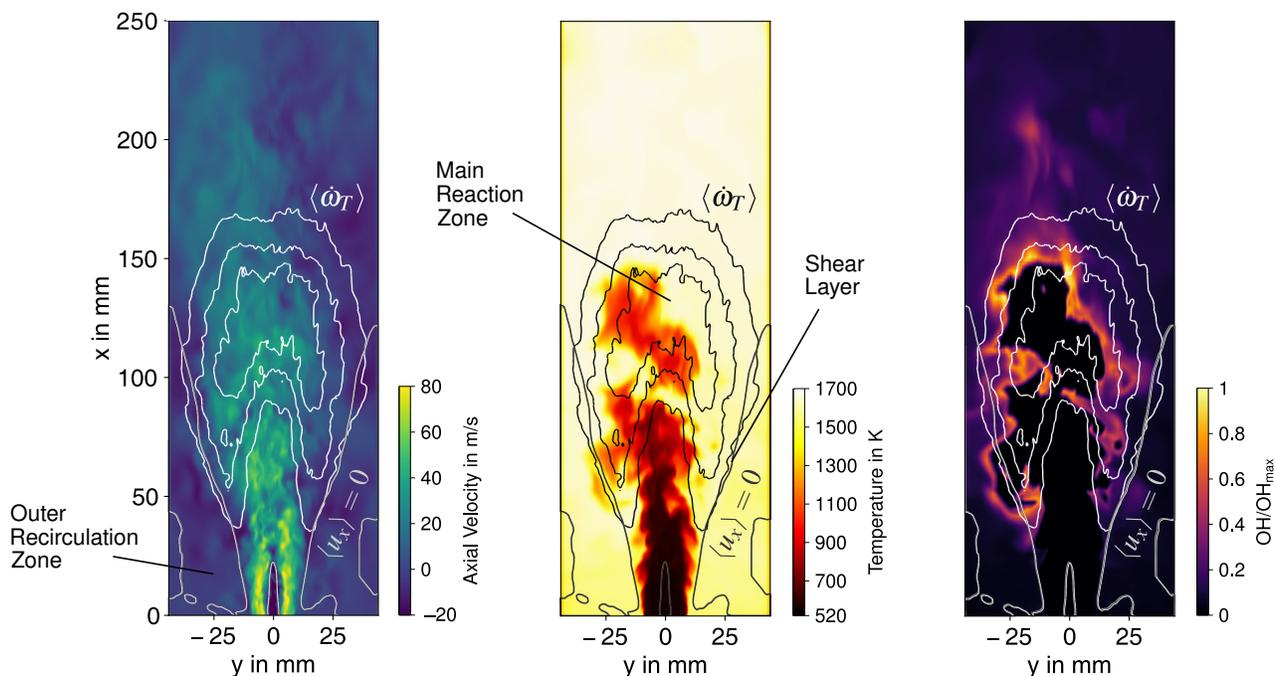
**FIGURE 5.** CONTOUR PLOTS OF THE INSTANTANEOUS FIELDS OF AXIAL VELOCITY (LEFT), TEMPERATURE (MIDDLE) AND OH MASS FRACTION (RIGHT) FOR THE SINGLE BURNER.
