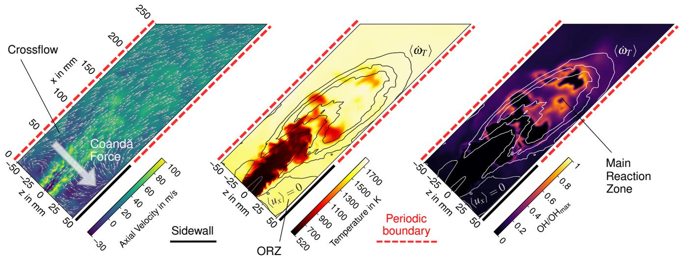
**FIGURE 8.** CONTOUR PLOTS OF THE INSTANTANEOUS FIELDS OF AXIAL VELOCITY (LEFT), TEMPERATURE (MIDDLE) AND OH MASS FRACTION (RIGHT) FOR THE SHC REFERENCE CASE. ARROW INDICATES THE DIRECTION OF THE DEFLECTING FORCE.
