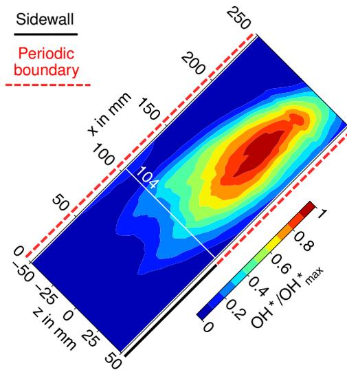
**FIGURE 9.** LINE-OF-SIGHT INTEGRATION OF THE  $\text{OH}^*$  MASS FRACTION FOR THE SHC REFERENCE CASE.
