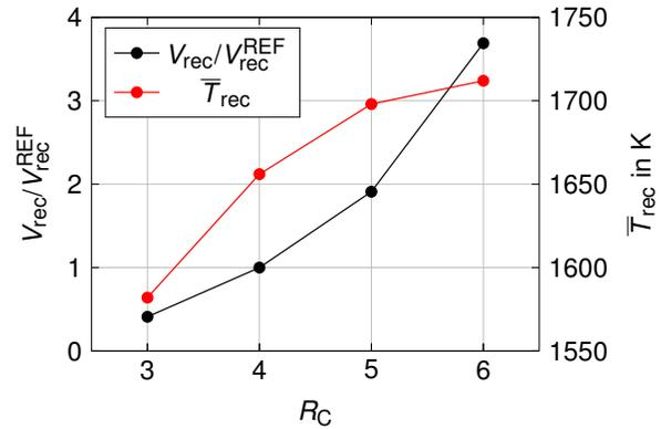
**FIGURE 11.** VOLUME AND VOLUME-AVERAGED TEMPERATURE OF THE OUTER RECIRCULATION ZONE OVER THE CONFINEMENT RATIO.
