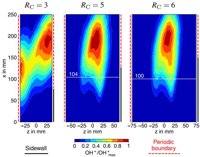
**FIGURE 12.** LINE-OF-SIGHT INTEGRATIONS OF THE  $\text{OH}^*$  MASS FRACTION FOR DIFFERENT CONFINEMENT RATIOS OF THE SHC.
