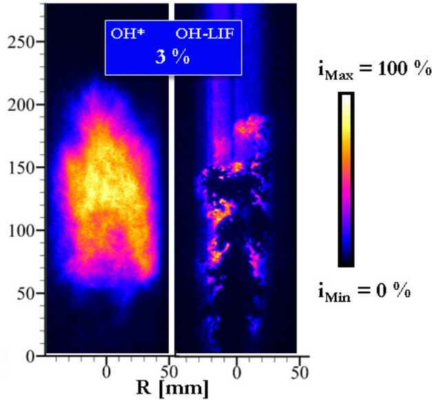
**FIGURE 3.** OH\* CHEMILUMINESCENCE AND PLANAR OH-LIF MEASUREMENTS ADAPTED FROM [26].
