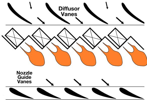
**FIGURE 1.** CONCEPTUAL SKETCH OF THE SHORT HELICAL COMBUSTOR ADAPTED FROM [12].
