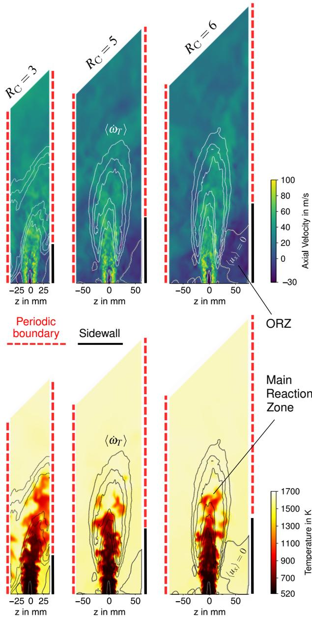
**FIGURE 10.** CONTOUR PLOTS OF THE INSTANTANEOUS FIELDS OF AXIAL VELOCITY (TOP) AND TEMPERATURE (BOTTOM) FOR DIFFERENT CONFINEMENT RATIOS OF THE SHC.
