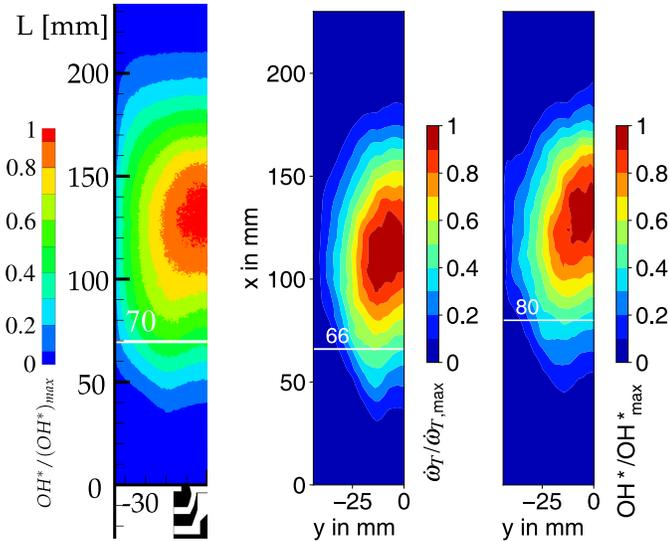
**FIGURE 6.** COMPARISON OF THE EXPERIMENTAL  $\text{OH}^*$  EMISSION INTENSITY (LEFT) ADAPTED FROM [26] TO THE LINE-OF-SIGHT INTEGRATIONS OF THE HEAT RELEASE (MIDDLE) AND  $\text{OH}^*$  MASS FRACTION (RIGHT).
