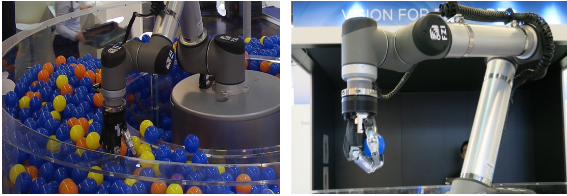
(a) The anthropomorphic hand catches a specifically coloured ball. (b) The robot's hand holding a ball, after a successful grasp.
