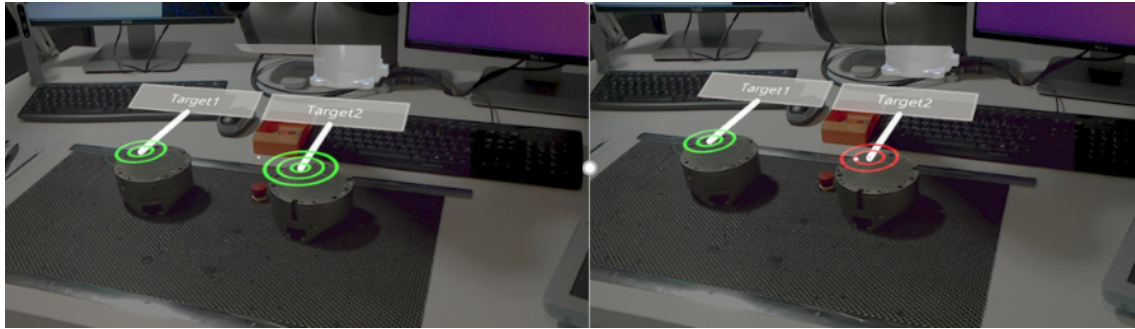
Figure 5.23: The current state of the workspace is displayed in AR. The information related to the workpieces state is represented with markers and text. Synthesized speech is used as well, in order to provide information about the robot target even if the user is not able to visually check the virtual overlay.
