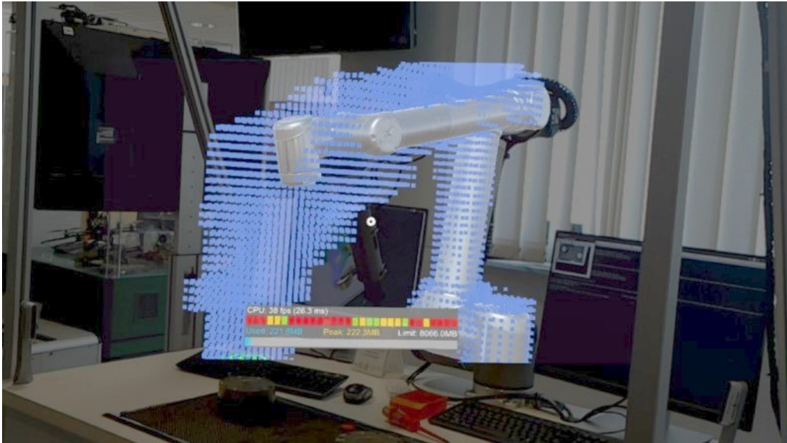
Figure 5.22: The point cloud representing the swept volume of the planned robot motion. This is used to predict collisions with the live environment and it is a useful information to understand the volume that the robot will occupy in the near future.
