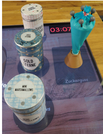
Figure 3.39: A set of control tools which can be used by the user to interact with the robot. Each one of them is identified and tracked by the Optitrack system through the use of different patterns of markers.
