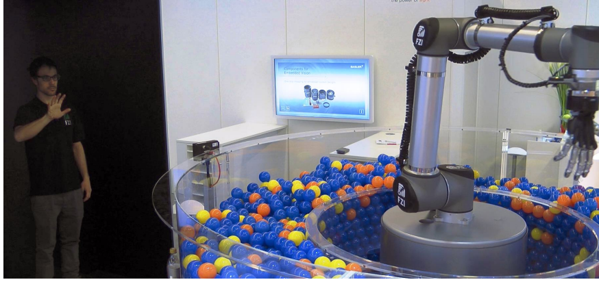
Figure 3.32: Claw crane game application. The user controls a 6 DOF robot equipped with an anthropomorphic hand, in order to grasp the desired prize.
