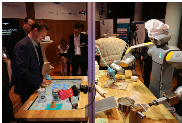
Figure 3.36: The user controls the robot TCP through the use of a tracked object. A graphical user interface guides the user in the interaction, enabling also a better precision in the control.
