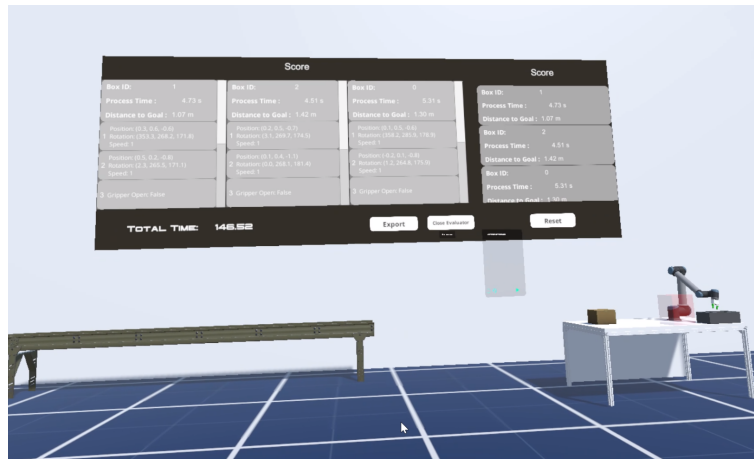
Figure 3.11: Once the three objects are successfully placed in the box, the metrics of the test are shown and stored. These include the overall time needed to perform the task, as well as the time needed by the robot to perform each pick and place operation.
