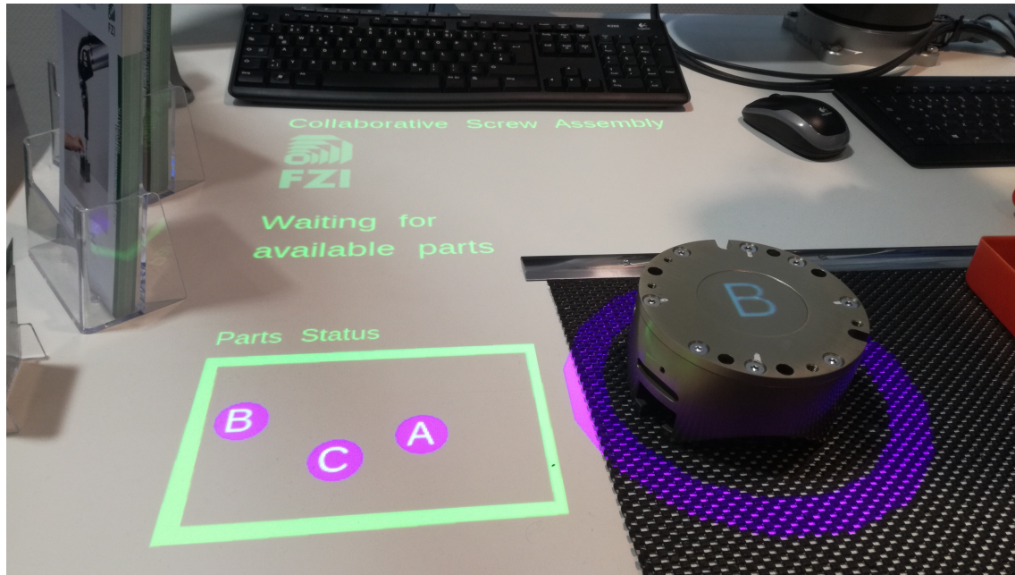
Figure 5.12: Text information on the side of the table allows the human to understand the status of the workpieces and the robot goal even if there are obstructions in the robot workspace.
