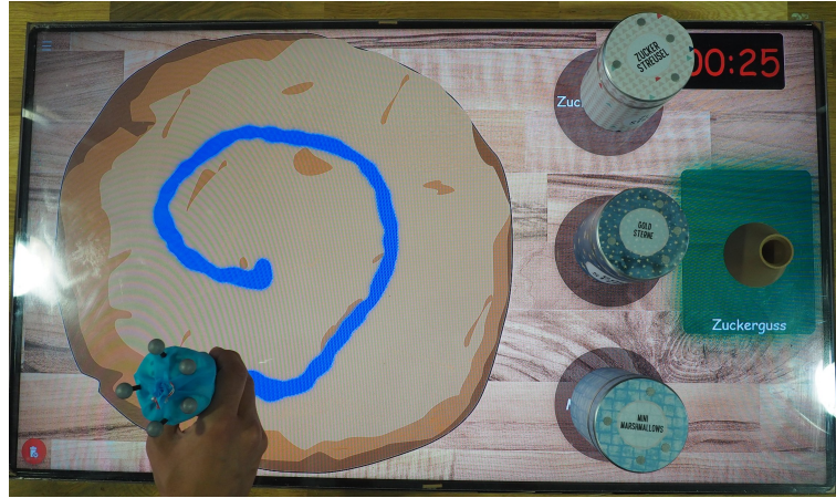
Figure 3.44: The GUI shows a simulation of the sugar flow that is dispensed through the tool. This is useful to give the user a feedback about the activation of the tool and help him in the definition of the desired path.
