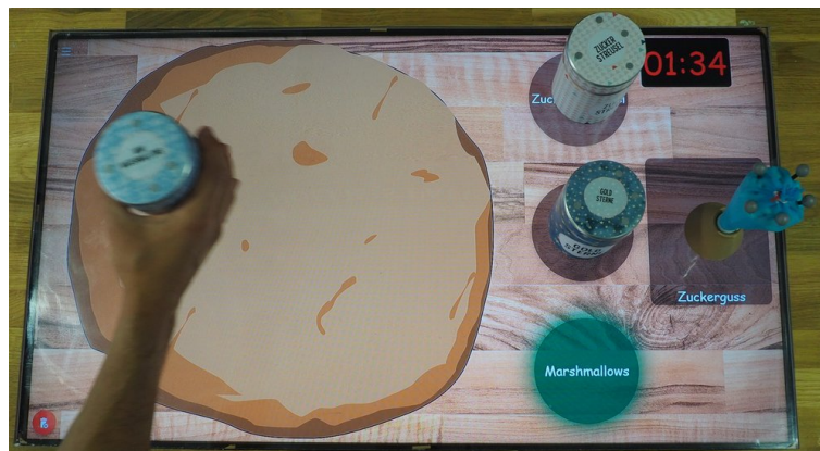
Figure 3.41: During the teleoperation mode, a scaled virtual representation of the object to be worked is displayed. This is useful to understand the control boundaries and to allow a better precision with the scaling of the motion. The GUI highlights also the current active tool and its placing position which is used to end the interaction or switch to another one.
