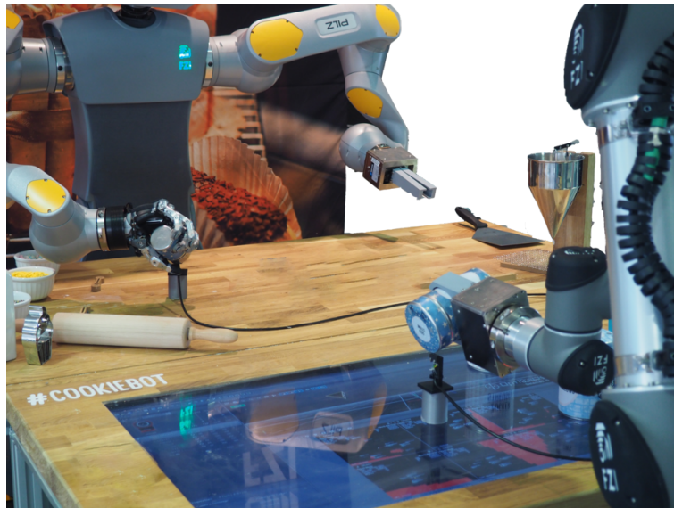
Figure 3.46: The setup used to evaluate the precision and motion latency of the system. A UR5 was used to move the tracked tool between different positions. The time needed to reach the different poses was measured with two buttons placed in the robots workspace.
