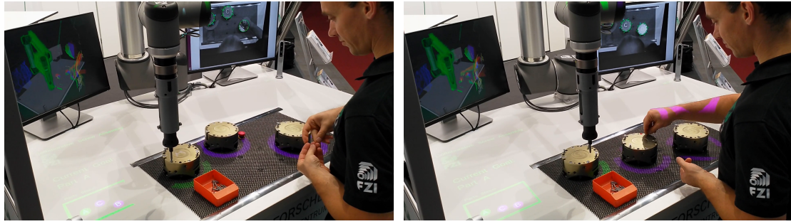
Figure 5.15: The user inspects the workspace and clearly understand the current target of the robot (a). The robot moves towards the user, but he is able to see that the target of the robot is still on the same workpiece (b). In this way he can continue to work without worrying about the robot motion.
