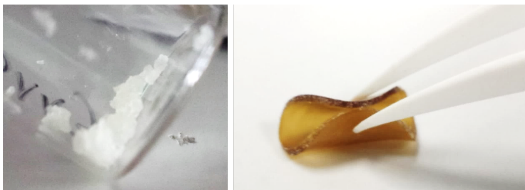
Figure 29: Pictures of crosslinked samples are given. The vial on the left contains a swellable gel out of a PAOMEC that was crosslinked using BMEE with 80% thiol per double bond. Samples with a lower crosslinker concentration did not form a stable solid. The picture on the right demonstrates the flexibility of a completely crosslinked polycarbonate network with PEO1000-dithiol as crosslinker.
