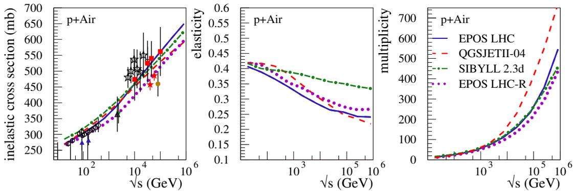
**Figure 2:** Inelastic cross-section (left-hand side), elasticity (energy fraction of the leading particle) (middle) and multiplicity (right-hand side) for p-air interactions as a function of center of mass energy. Simulations are done with EPOS LHC-R (dotted line), EPOS LHC (full line), QGSJETII.04 (dashed line), and SIBYLL 2.3d (dash-dotted line). Points are data from [20].
