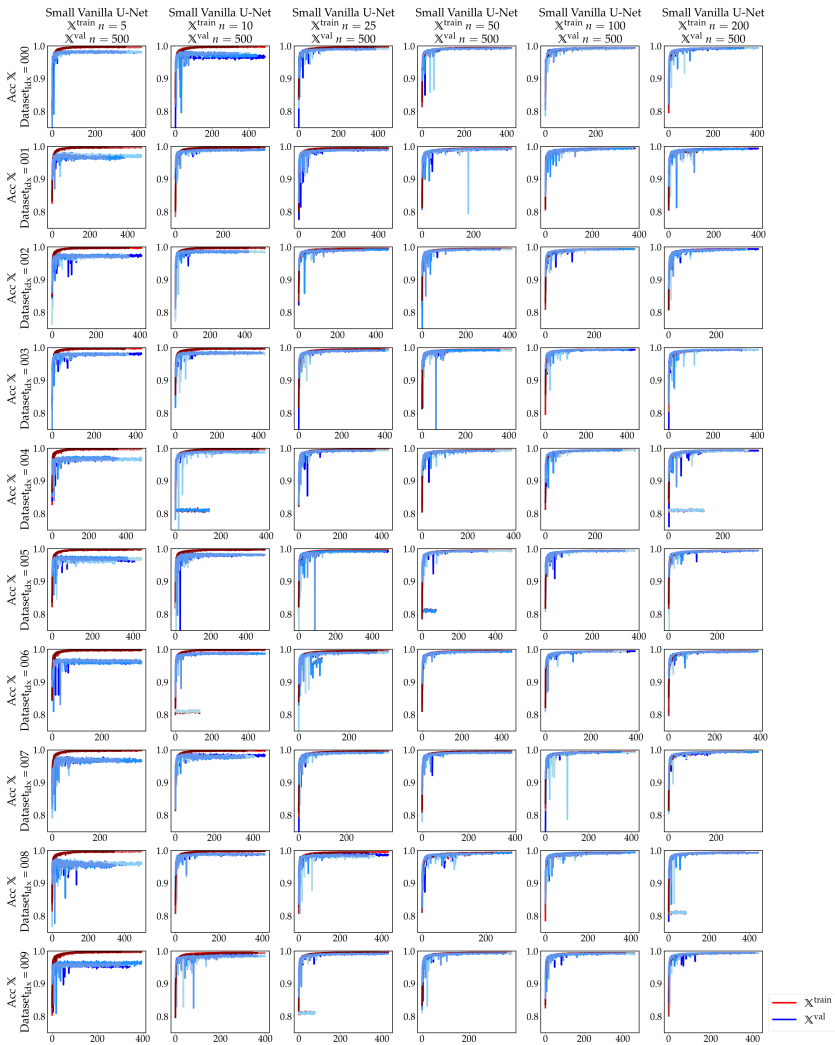
Figure A.3 Accuracy of the small vanilla U-Net. In red are the results on the data set \mathbb{X}^{\text{train}} and in blue for \mathbb{X}^{\text{val}} . The x-axis represents the progression of epochs during the training process. Five model were trained on each data split from scratch.
