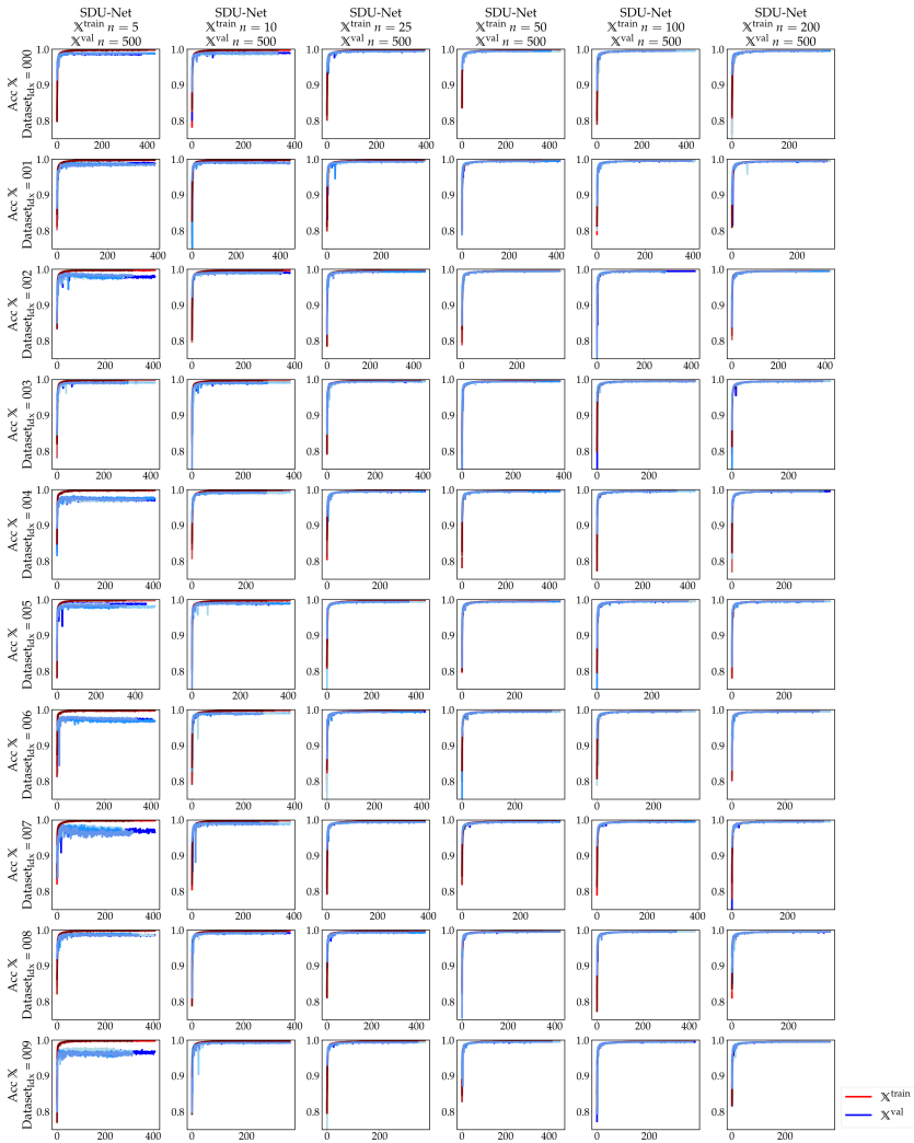
Figure A.5 Accuracy of the SDU-Net. In red are the results on the data set \mathbb{X}^{\text{train}} and in blue for \mathbb{X}^{\text{val}} . The x-axis represents the progression of epochs during the training process. Five model were trained on each data split from scratch.
