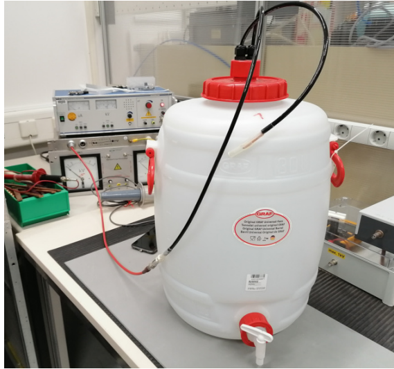
Figure 43 High voltage test of 4 m SC-Aqua Marinex coaxial cable submerged in water.
