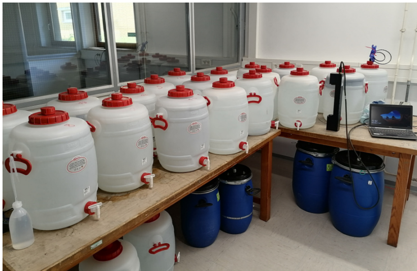
Figure 46 Measuring station for the water quality measurement with the samples stored in barrels. The transmissometer stands next to the notebook.
