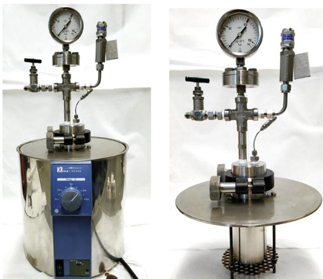
**Figure 2.** Setup for hydrothermal synthesis of nanostructured Nb<sub>2</sub>O<sub>5</sub> with niobium ammonium oxalate.
