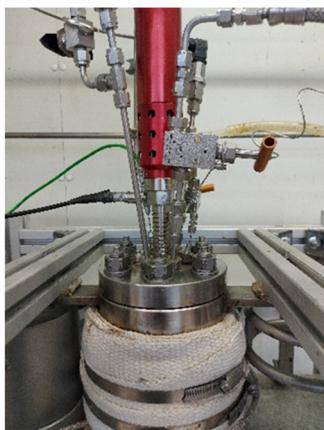
**Figure 3.** Batch reactor for HDO tests.
