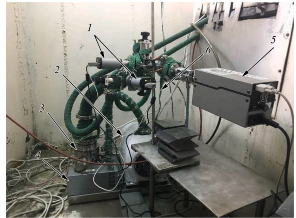
Fig. 3. The part of the CIRRA facility in the experimental box: 1 – pressure sensors; 2 – spiral pump; 3 – turbomolecular pump; 4 – controller of turbomolecular pump; 5 – mass spectrometer; 6 – heating tape.
