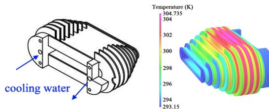
Figure 6: Left: the design of the coil former with built-in cooling channels [10]; right: heat analysis model of the coil in OPERA in full excitation.
