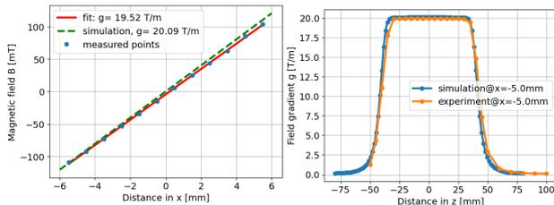
Figure 9: Transverse and longitudinal magnetic measurement results at operating current of 1 A.
