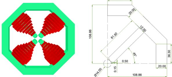
Figure 2: Magnet OPERA 3D model and dimension in mm.
