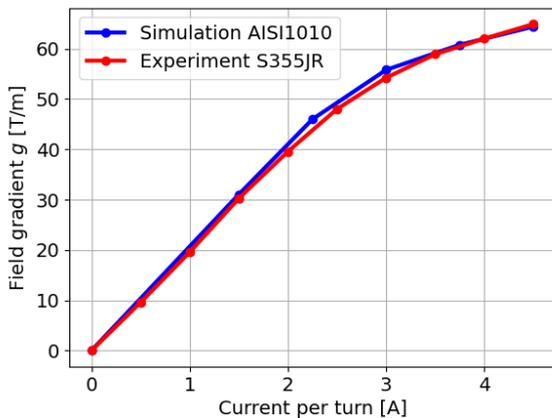
Figure 8: Field gradients as a function of operating currents comparison of materials AISI1010 (simulation) and S355JR (experiment).
