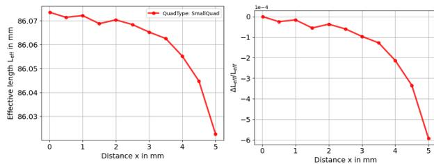
Figure 5: Left: effective length within GFR; right: relative deviation of effective length within GFR.
