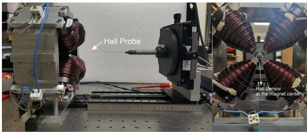
Figure 7: Left: experiment setup for the magnetic measurement of the first prototype; right: the measuring point at the center of the magnet
