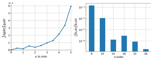
Figure 4: Left: absolute integrated field quality in the longitudinal direction; right: integrated normalized multipole errors of the chamfered model at 5 mm.
