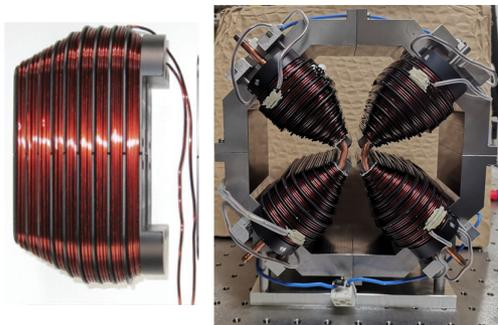
Figure 3: Coil [5] and the first prototype of the quadrupole without cooling system.
