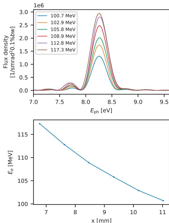
Figure 5: Photon flux density over photon energy calculated using the measured field maps, scaled to nominal operating current (750 A). The simulation assumes zero-emittance electron beamlets with a beam current of 10 pA, traveling through the TGU at the reconstructed Hall probe positions. The bottom panel shows the according spectral dispersion, resulting from an optimization of the electron energies for a monochromatic photon spectrum.
