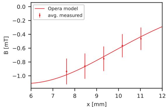
Figure 3: Magnetic flux density generated by the correction coils, averaged over the scanning range, as a function of reconstructed transverse position. The measured data are compared to an Opera-3D simulation.
