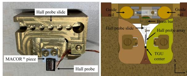
Figure 1: Left: Part of the brass slide with Hall probe array mounted. Right: cross-sectional view of the TGU with magnetic measurement system.
