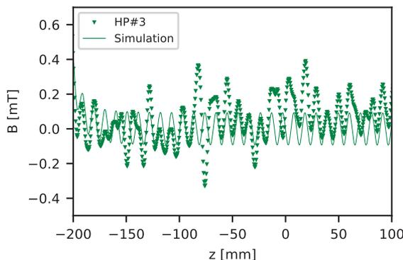
Figure 4: Magnetic flux density generated by the TGU, averaged over a rolling window spanning over one period length, corresponding residual net kicks to the beam along its trajectory. The data are shown for all full TGU periods in the scanning range (excluding the matching periods).
