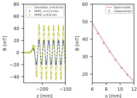
Figure 2: Magnetic flux density  $B_{\perp}$  at TGU operating current  $I_{op} = 30$  A, comparison of measured data with Opera-3D simulation for the first periods as function of  $z$  (left) and amplitude average over all periods as function of  $x$  (right).
