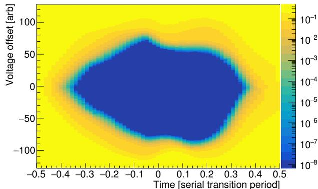
Figure 2: Eye diagram representing the Bit Error Rate (BER) as a function of the time from the zero crossing and Voltage offset as measured on the Xilinx Versal VCK190 Breakout Board with a 14 Gbps FireFly™ FMC Development Kit at 10 Gbps.
