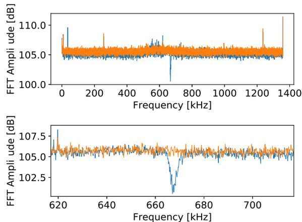
Figure 4: Comparison of BPM signal FFT with the feedback (blue line) and without beam (orange line). The notch produced by the feedback is clearly visible. The lower plot shows a zoom in the notch region. The peak in the 30 kHz region (blue line) is due to synchrotron oscillations.
