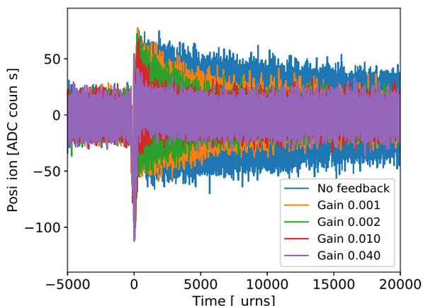
Figure 3: Position measured with the BPMs as a function of time, expressed in turns, for different gains of the feedback system. The injection kick arrives at  $t = 0$ .
