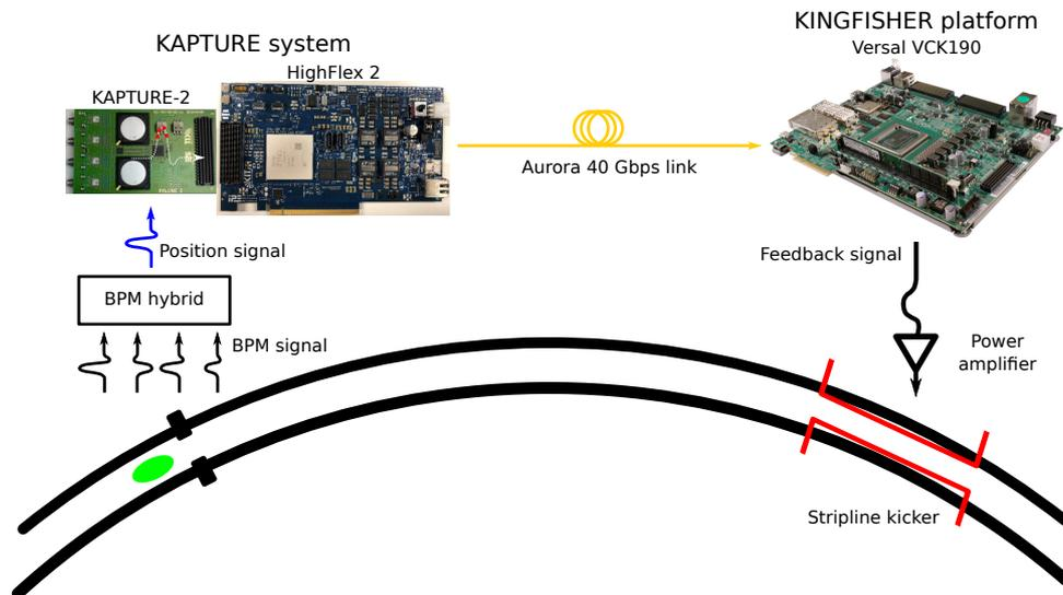
Figure 1: Schematic drawing of the feedback loop implemented at KARA, showing the main electronic boards used.
