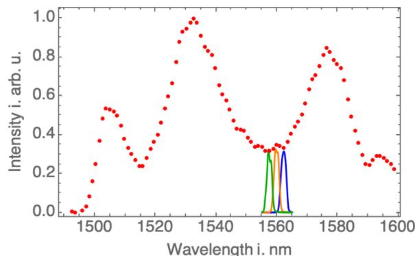
Figure 3: Shown is a graph with single measurements (green, yellow, blue) using the described setup using a slit and a collimator and the maxima of fits to all single measurements plotted with red dots reproducing the spectral shape.
