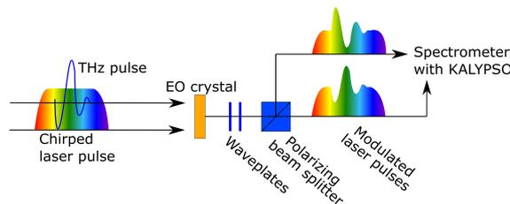
Figure 1: Schematic of the EOSD setup using balanced detection [4].
