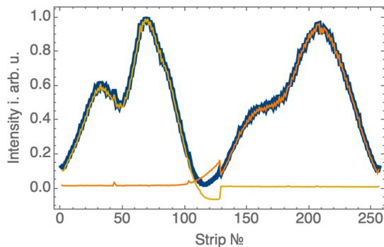
Figure 5: Shown are the intensities detected with KALYPSO plotted against the strip number. The measurement with two beam spots (thick blue line) is overlaid with two further measurements (yellow, orange) where one beam path was blocked.
