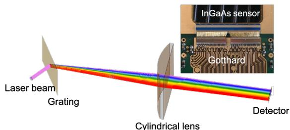
Figure 2: Illustrated is the simulated beam path including the optics (grating and cylindrical lens) as well as a photo of the sensor part or KALYPSO (InGaAs sensor) with the Gotthard chips.
