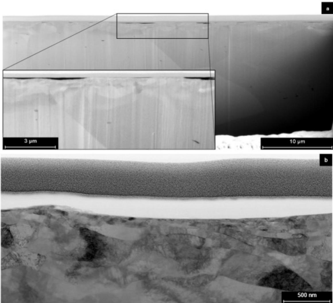
Figure 4.16: Images of cross sections cut perpendicular to the sliding direction in the middle of the wear track after microtribometer experiments at  $3.5\ \mu\text{m}$  thickness and  $402\ \text{mN}$  yielded by (a) SEM and (b) bright field TEM. From [79].
